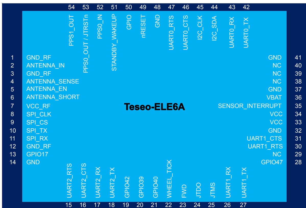
Figure 2. Module pins layout
