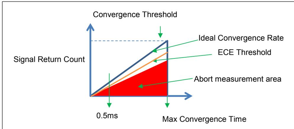
To expand on the ECE factor, if the user chooses an 80% ECE factor, the resulting ECE threshold result is shown in Figure 3 below. What this means is that the system will gather the return signal count and if these are above 80% of the ideal convergence rate after 0.5ms of the measurement starting then the system will allow the measurement to continue.
