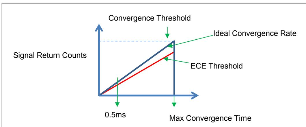
To give another ECE factor example, if the user chooses a 110% factor, the resulting ECE threshold result is shown in Figure 4 below. What this means is that the system will gather the return signal count and if these are above 110% of the ideal convergence rate after 0.5ms of the measurement start, then the system will allow the measurement to continue.
