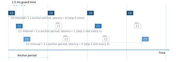
Figure 4. Example: setting Latency = 0, 1 or 2 for CONN slots
