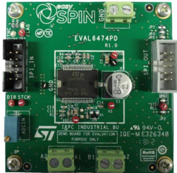
Figure 1. EVAL6474PD evaluation board
