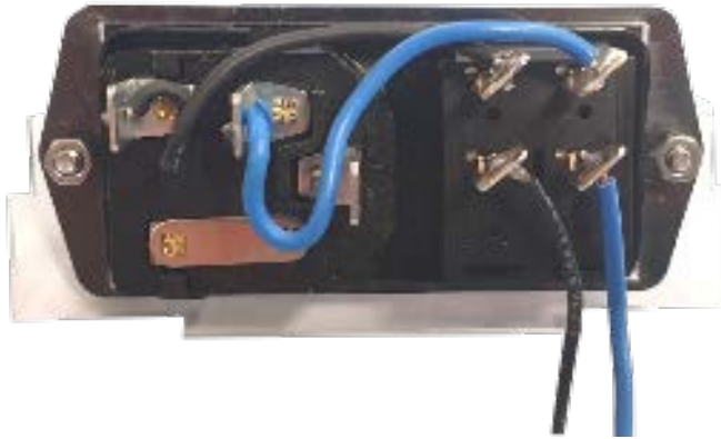
Figure 5. Mounting the IEC connector (1 of 2)
