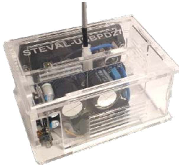
Figure 11. Mounting the STEVAL-USBPD27S in the shroud (5 of 5)
