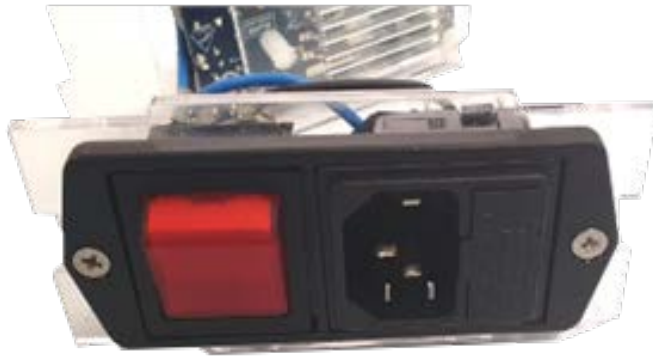
Figure 6. Mounting the IEC connector (2 of 2)
