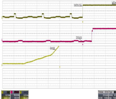
Figure 1. T2P not asserted. Note the VDD rise that is monotonic. This picture is obtained removing the classification resistance
