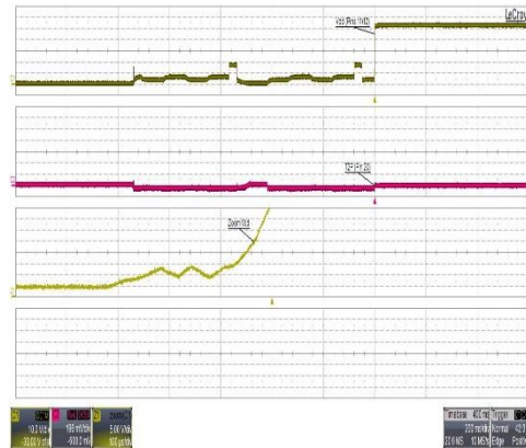
Figure 2. Same PD with Class 4: The T2P is asserted. Note the VDD rise that is not monotonic, but has for two times a negative slope, clear indication that the switch port is in current limitation.
