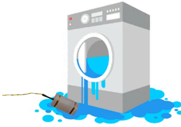
Figure 5. Example of application. The probe is positioned under a washing machine to detect water leakage.
