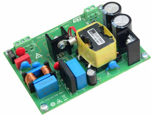
50 W converter based on HVLED101 quasi-resonant HPF flyback controller with secondary-side regulation ( EVLHV101SSR50W )
