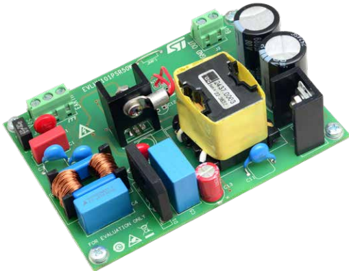
50 W converter based on HVLED101 quasi-resonant HPF flyback controller with primary-side regulation ( EVLHV101PSR50W )
