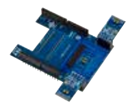
P/N: X-NUCLEO-53L3A2 Multi-targets VL53L3CX ranging sensor expansion board
