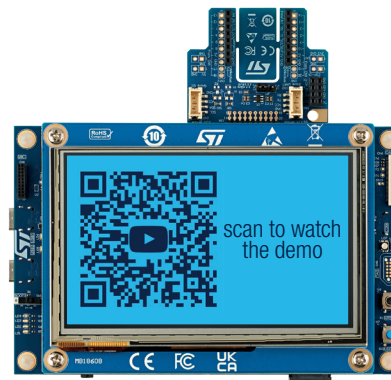
STM32H7S78-DK Essential prototyping 256-Mbit Octo-SPI NOR Flash, Ethernet, USB, Stlink debugger, Arduino UNO extension interface.
