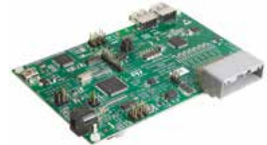
L9963E evaluation board (EVAL-L9963E-MCU) with on-board SPC5 MCUs and preloaded firmware
