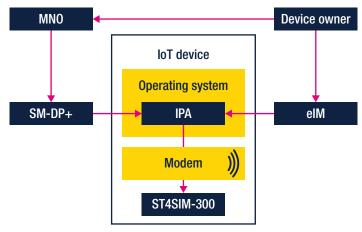
eSIMs allow remote swapping of operators without physical access. The device owner establishes an agreement with the selected mobile network operator (MNO) and triggers the profile download process through the eSIM for IoT remote manager (eIM). This new architecture significantly simplifies the process of swapping operators for device owners.
