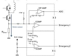
The number of external components required to implement these functionalities can be reduced using a microcontroller that embeds such peripherals. STMicroelectronics' portfolio includes the STM32F30x family that contains up to four programmable gain amplifiers and up to seven fast comparators glued in the architecture design specifically for motor control applications.
