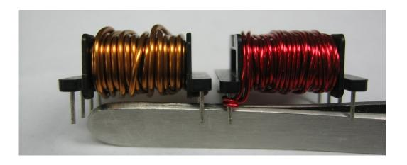
The coil on the right uses a two-bi winding to achieve the same DC resistance, but better layering.
