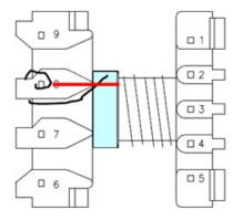
**Triple Insulated Wire on SEC to insulate windings**
