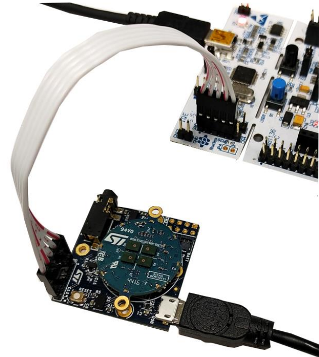
SWD connections with 5-pin flat cable
