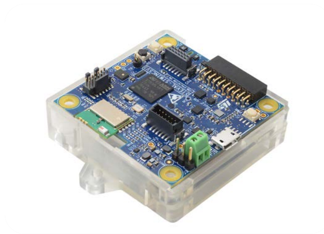
STWIN Industrial node with ISM330DHCX
