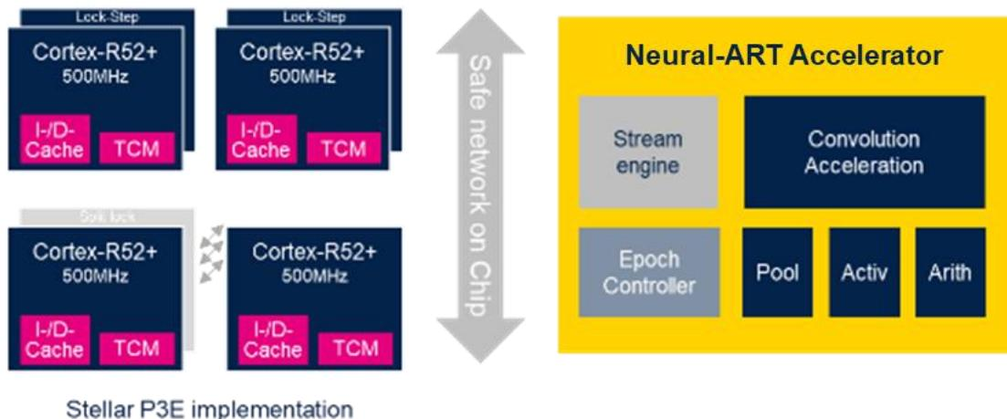
**Neural-ART Accelerator:** ST proprietary neural processing unit (NPU) with **data-flow architecture** optimized to run neural network models **efficiently**.
