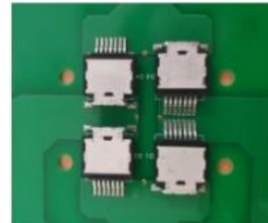
Figure 7. HU3PAK sample mounted on test PCB
