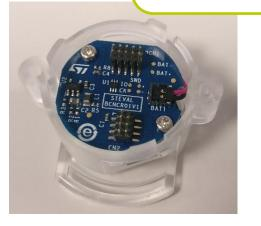
the cradle, insert in the plastic case and secure with the bolts
