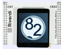
RVA15MD-NUC64A NUCLEO64 extension display from Riverdi 1.5" PCAP touch IPS display
