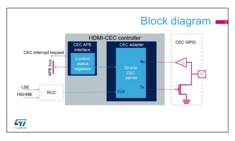
HDMI-CEC stands for "High-Definition Multimedia Interface" - "Consumer Electronics Control". The controller complies with HDMI-CEC v1.4 specifications. It provides functions needed to interface with various audiovisual products.
