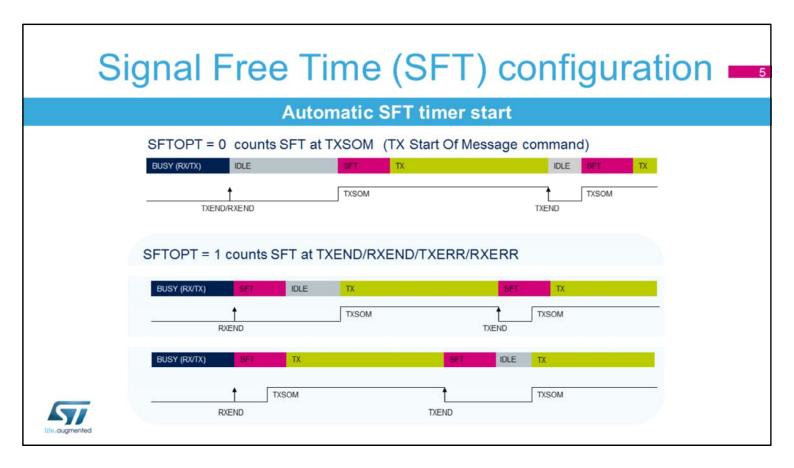
When a transmit command is sent, the HDMI-CEC sends a Start bit after the following number of nominal data bit periods of inactivity which depends on the programmed Signal Free Time (SFT) value.
