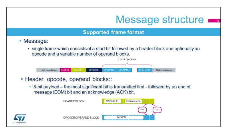
The supported frame format consists of a start bit followed by a header block and optionally an opcode and then a variable number of operand blocks.
