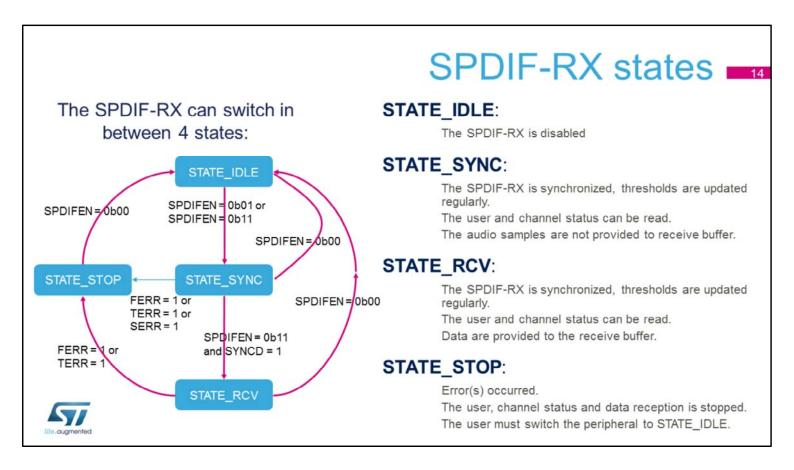
The figure shows the different states of the SPDIF-RX. The state of the SPDIF-RX can be changed by the application, via the field SPDIFEN or by the SPDIF-RX hardware mainly if errors are detected.
