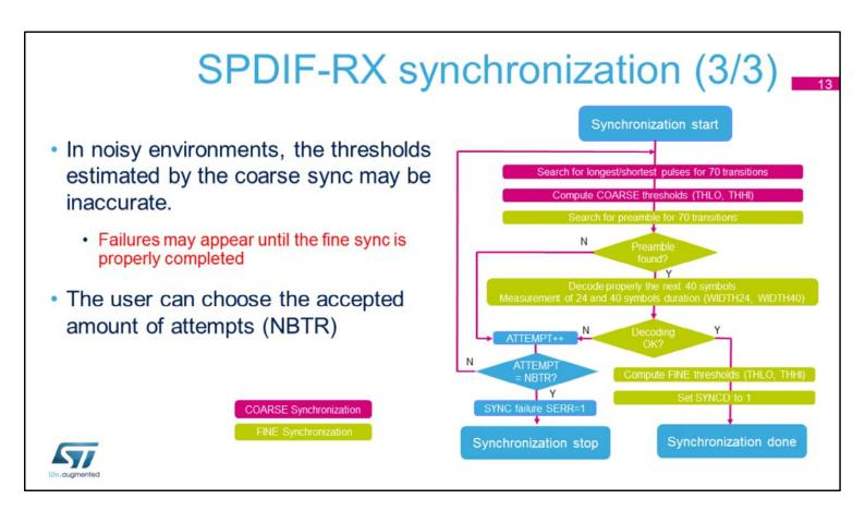
The figure shows the hardware process performed by the SPDIF\_RX in order to estimate properly the THLO and THHI thresholds.
