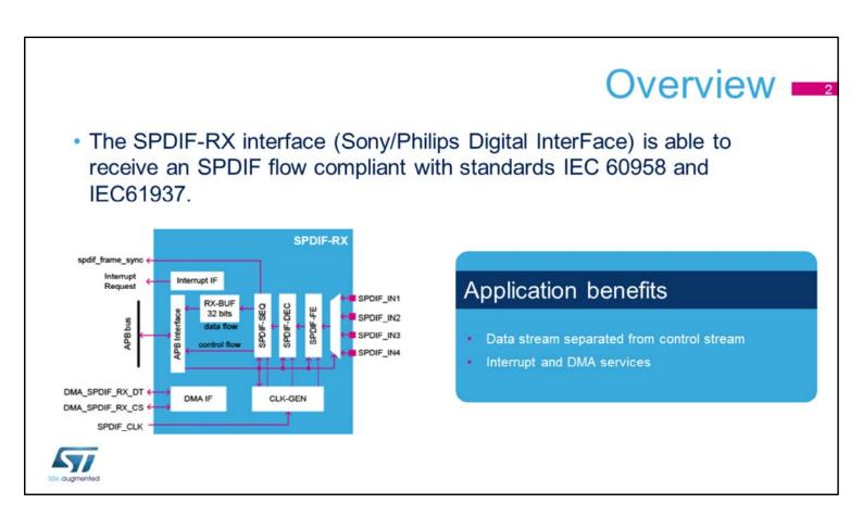
The SPDIF-RX block is able to receive digital audio streams compliant with the IEC-60958 and IEC-61937 standards.
