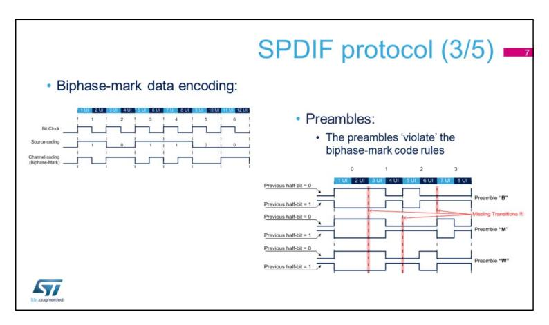
The digital audio data are coded using biphase-mark encoding as shown in the upper figure.
