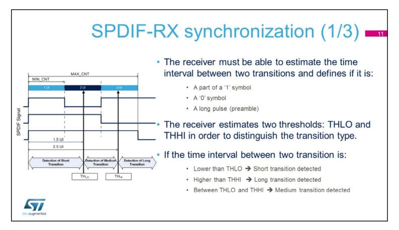
In order to decode the incoming stream, the SPDIF-RX estimates the duration of one UI and defines two thresholds:
