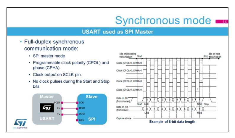
The USART can also communicate synchronously. It can operate as a SPI in Master mode with programmable clock polarity (CPOL) and phase (CPHA). The clock is output on the SCLK pin. No clock pulses are provided during the start and stop bits.
