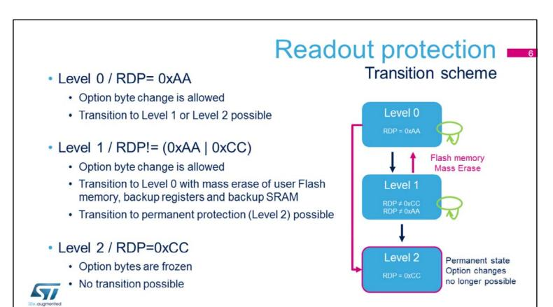
This slide shows the possible transitions between each readout protection level. It is always possible to raise the protection level but regression is only possible between Level 1 and Level 0 with the consequence of a full User Flash Erase operation.
