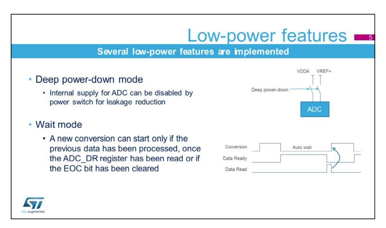
The ADC supports a Deep power-down mode. When the ADC is not used, it can be disconnected by a power switch to further reduce the leakage current. When Wait mode is active, the ADCs wait until the last conversion data is read or the end-of-conversion flag is cleared before starting the next conversion. This avoids unnecessary conversions and thus reduces power consumption.
