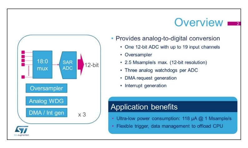
The analog-to-digital converter inside the STM32G0 microcontroller allows the microcontroller to accept an analog value like from a sensor output and convert the signal for use in the digital domain. There are up to 19 analog inputs. The ADC module itself is a 12-bit successive approximation converter with additional oversampling hardware.
