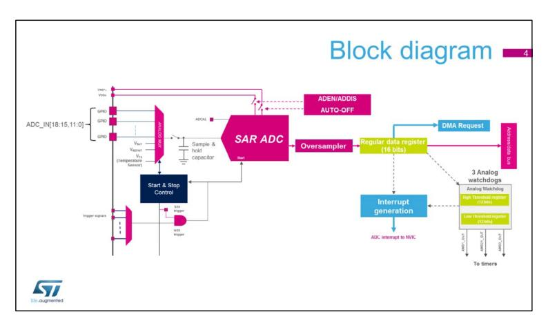
This slide shows the general block diagram of the ADC. The left part describes the analog front-end, based on the analog multiplexer and the embedded sampling capacitor of the ADC. This sampling time must be enough for the input voltage source to charge the sample and hold capacitor to the input voltage level.
