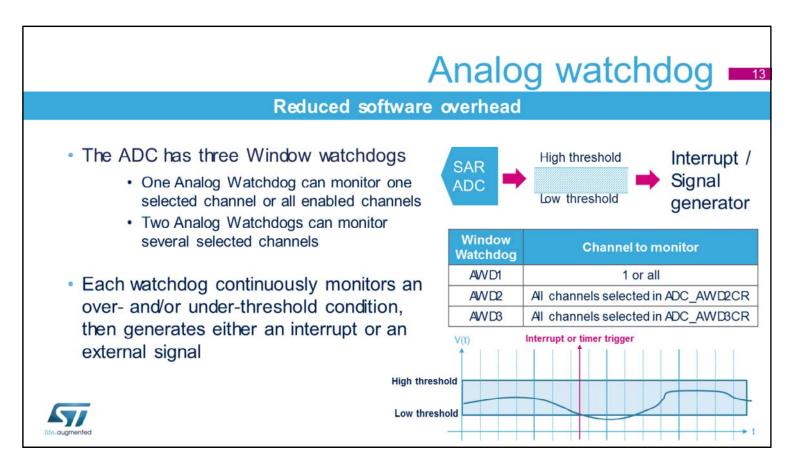
Each ADC has 3 integrated 12-bit analog watchdogs with high and low threshold settings. The ADC conversion value is compared to this window threshold, if the result exceeds the threshold, an interrupt or timer trigger signal can be asserted without CPU intervention.
