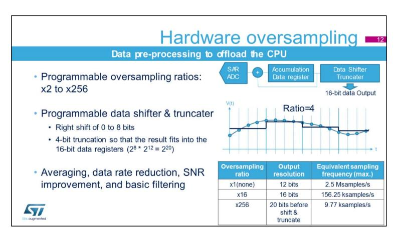
The ADCs support hardware oversampling. They can sample by 2 to 256 times without CPU support. The converted data is accumulated in a register and the output can be processed by the data shifter and the truncater.
