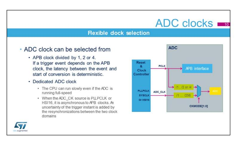
The ADC has a selectable clock source. When the system needs to run synchronously, the APB clock source is the best selection. If a slow CPU speed is required, but the ADC needs a higher sampling rate, the dedicated ADC clock can be selected. In this case, the ADC implements two clock domains: PCLK and ADC\_CLK and delays are needed to perform the resynchronizations between them.
