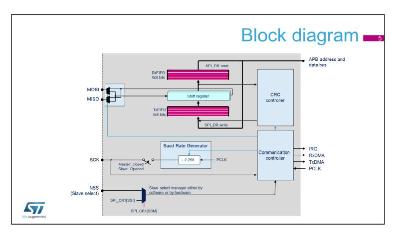
The simplified SPI block diagram shows its basic operation and functions. There are four I/O signals associated with the SPI peripheral. All data passes through the receive and transmit buffers via their specific interfaces.
