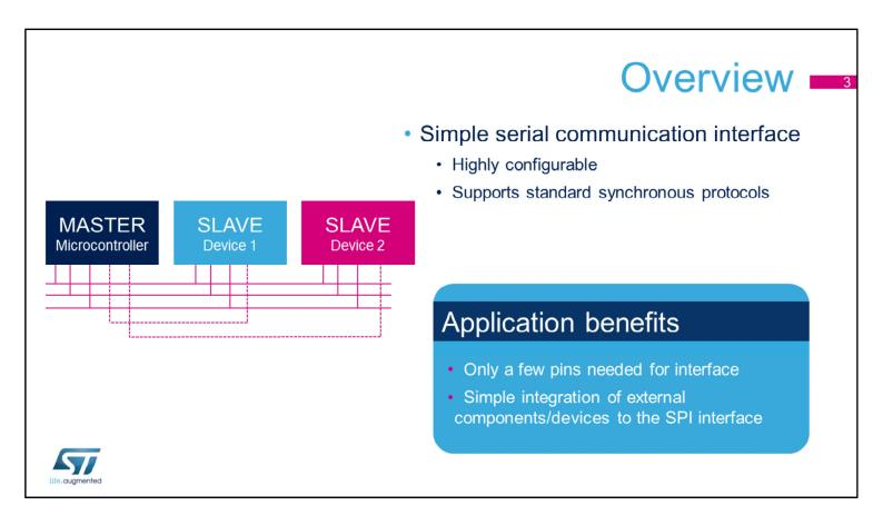
The internal Serial Peripheral Interface or SPI provides a simple communication interface allowing the microcontroller to communicate with external devices. This interface is highly configurable to support many standard protocols.
