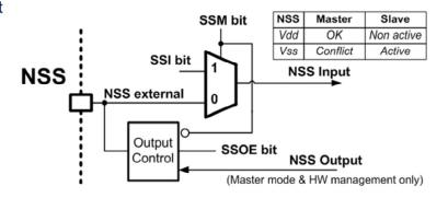
The Slave Select signal is commonly used by the master node to select the slave node for communication.
