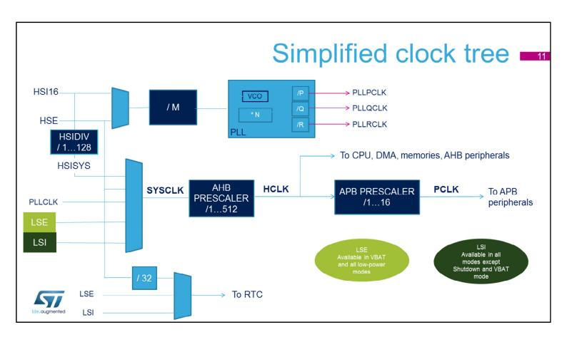
The system clock can be derived from the high-speed internal 16 MHz RC oscillator (HSI16), the high-speed external 4 to 48 MHz oscillator (HSE), the low-speed internal oscillator (LSI) or the low-speed external oscillator (LSE). The AHB clock, called HCLK, is derived by dividing the system clock by a programmable prescaler. The APB clock, called PCLK is generated by dividing the AHB clock by a programmable prescaler.
