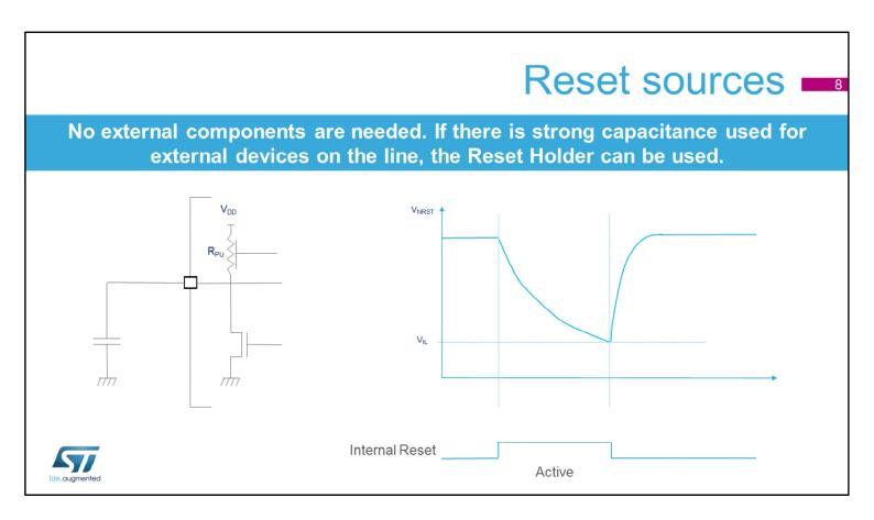
The purpose of the reset holder is to maintain NRST driven LOW until the voltage level of this signal goes below VIL. This is useful when the NRST line has an important capacitive load.
