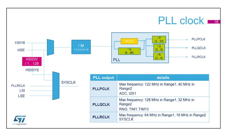
STM32G0 devices embed a phase-locked loop, each with 3 independent outputs. The input clock of the PLL can be selected between HSI16 and HSE.
