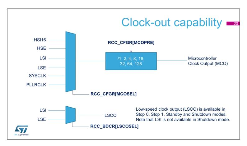
The various clocks can be output on an I/O. The Microcontroller Clock Output feature allows you to output on a pin one of these six clocks, HSI16, HSE, LSI, LSE, SYSCLK, and PLLCLK.
