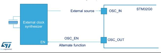
In External source mode, also called HSE bypass mode, an external clock source must be provided. It can have a frequency of up to 48 MHz.
