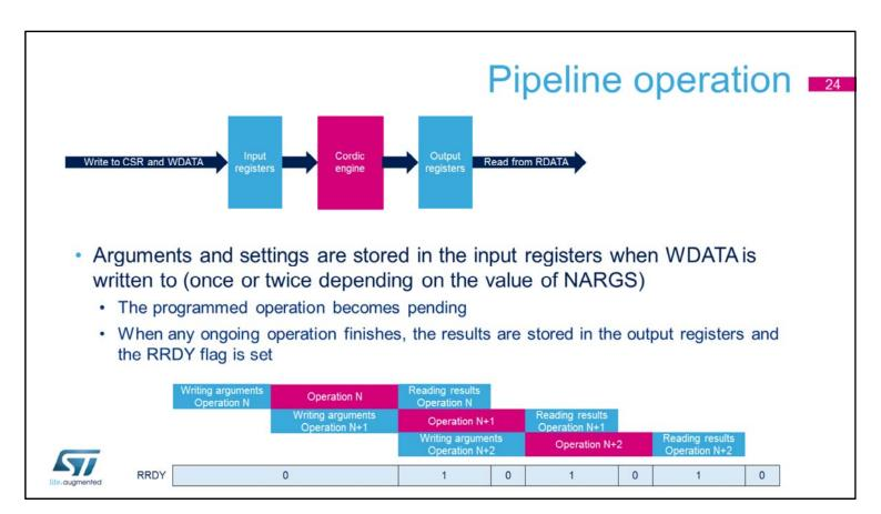
As soon as the results have been read from RDATA (one or two reads depending on the value of NRES), the pending operation is started.
