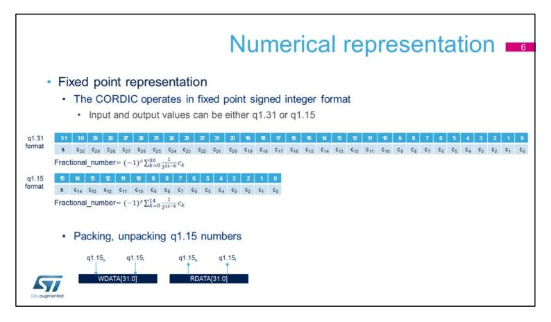
In q1.31 format, numbers are represented by one sign bit and 31 fractional bits (binary places).
