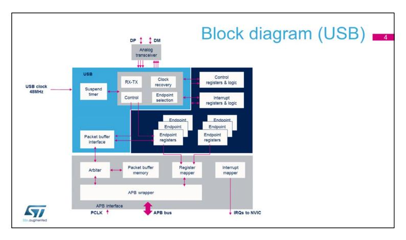
The block diagram of the USB Full Speed device controller shows the various building blocks inside along with its analog transceiver, which manages the physical layer, shown above.
