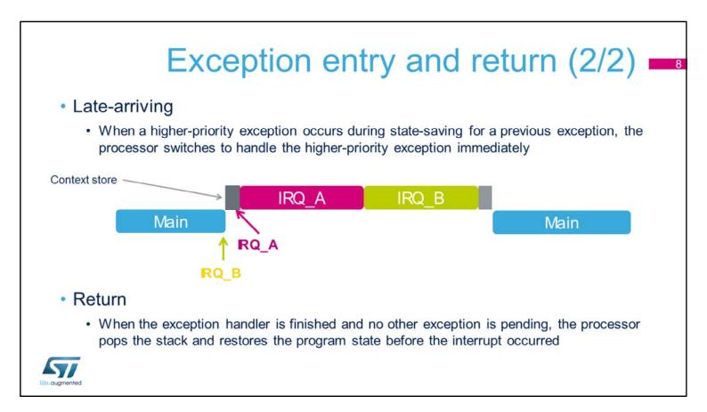
When an interrupt arrives, the processor first saves the program context before executing the interrupt handler. If the processor is performing this context-saving operation when an interrupt of higher priority arrives, the processor switches directly to handling the higher-priority interrupt when it is finished saving the program context. Then tail-chaining will be used prior to executing the IRQ\_B interrupt service routine.
