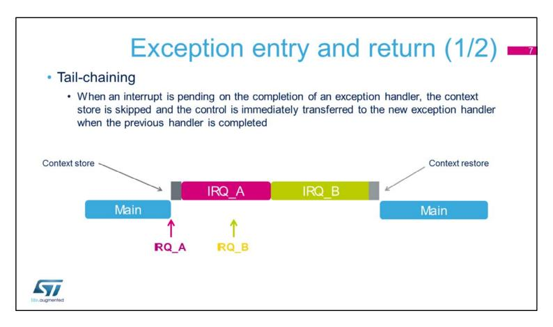
When an interrupt request with lower or equal priority is raised during execution of an interrupt handler, it becomes pending. Once the current interrupt handler is finished, the context saving and restoring process is skipped and control is transferred directly to the new exception handler to decrease interrupt latency. So back-to-back interrupts with decreasing priorities (higher priority values) are chained with a very short latency of a few clock cycles.
