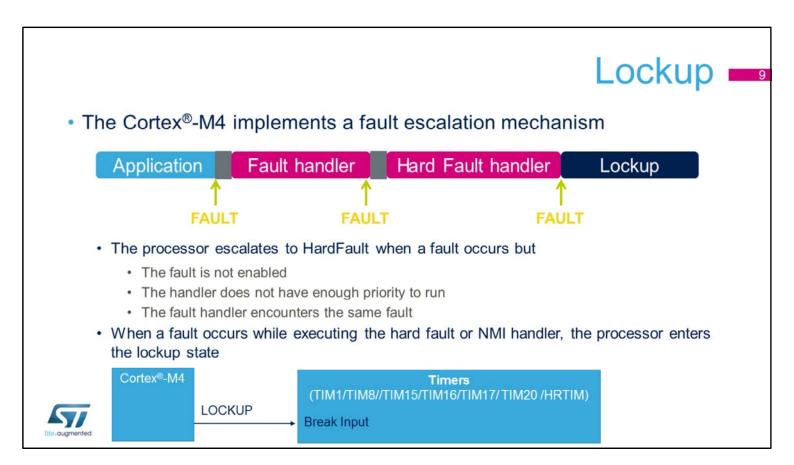
When a fault occurs while executing either the bus fault handler or the memory management fault handler or the usage fault handler, the processor escalates this event to the hard fault handler.
