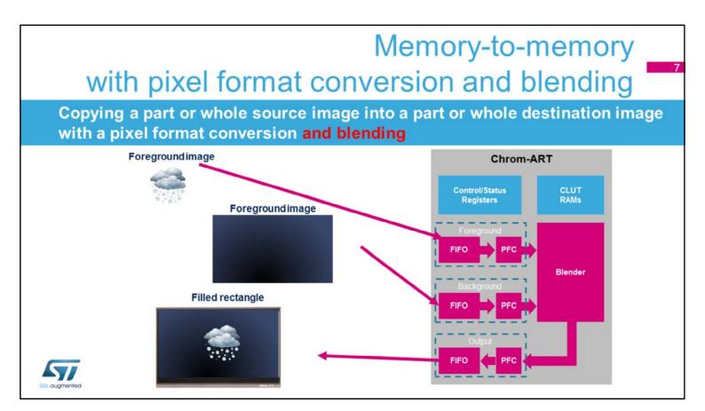
Memory-to-memory mode with pixel format conversion and blending is used to blend a part or whole source image with a part or whole destination image with a different pixel format. This is widely used to draw bitmap icons having transparency or fonts.
