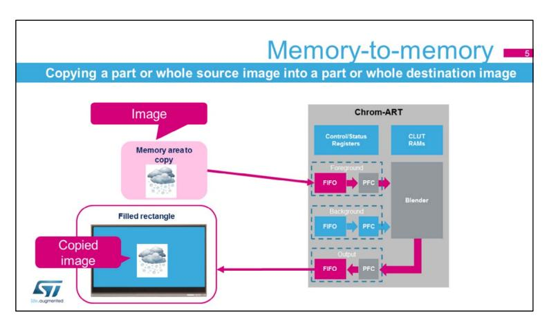
Memory-to-memory mode is used to copy a part or whole source image into a part or whole destination image without changing the color format.
