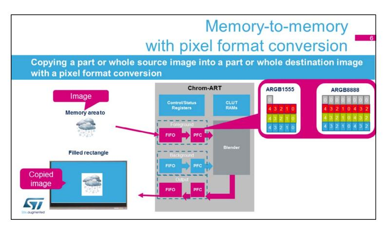
Memory-to-memory mode with pixel format conversion is used to do the same type of copy as Memory-to memory mode but with a pixel format conversion. It can copy any input format to any output format. For example, it can copy an ARGB565 image into an ARGB888 image without having to use the CPU.
