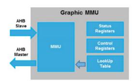
The Graphic MMU is a graphical oriented Memory Management Unit aimed to optimize memory usage according to the display shape (ex. round display).
