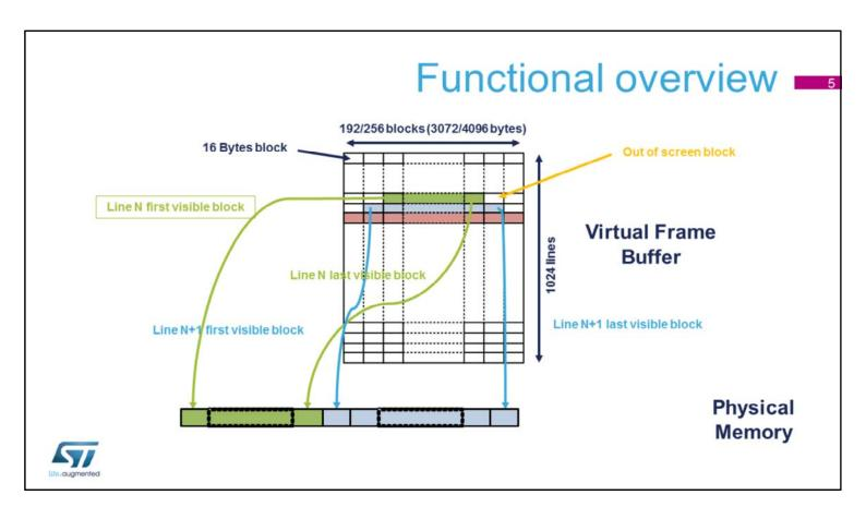
The operation is repeated for each line, indicating the first block and the last block.
