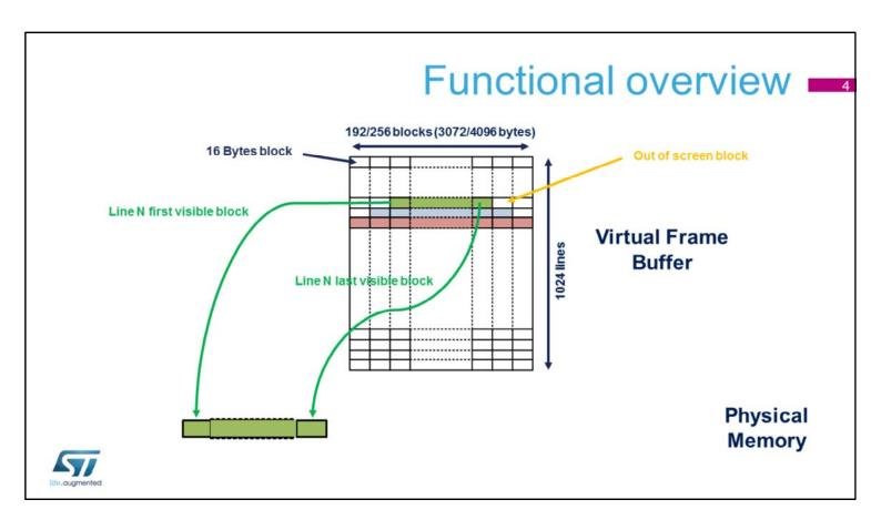
Each virtual buffer is seen as a continuous memory space of 3072 or 4096 bytes per 1024 lines.
