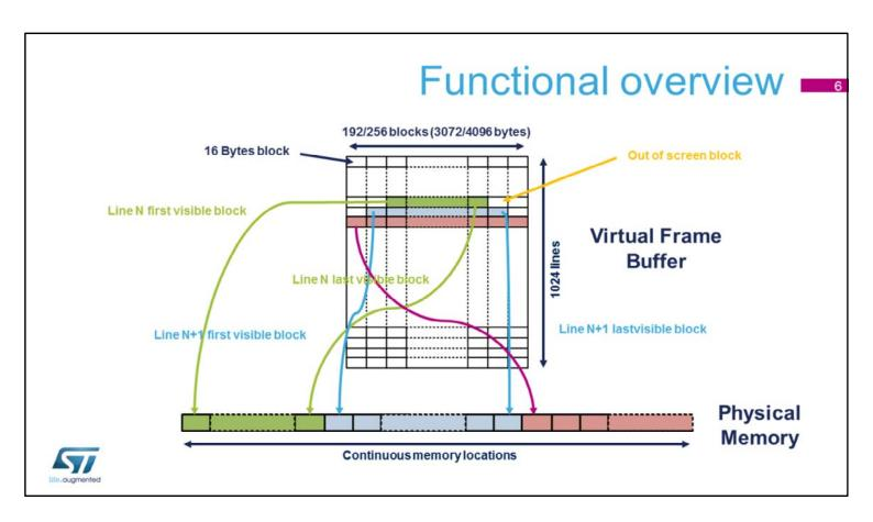
And all the visible blocks are stored in the physical memory in a continuous way saving a huge amount of space for non-rectangular display shapes.
