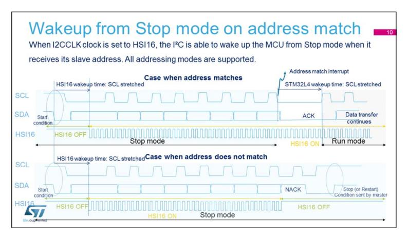
The I<sup>2</sup>C peripheral supports Wakeup from Stop mode on address matches. To do this, the I<sup>2</sup>C peripheral clock must be set to the high-speed internal 16 MHz RC oscillator. Only the analog noise filter is supported when the Wakeup from Stop feature is enabled. All addressing modes are supported.
