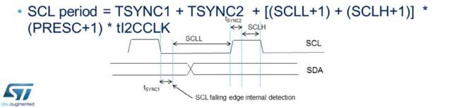
The I<sup>2</sup>C master clock's low- and high-level durations are configured by software in the I<sup>2</sup>C Timings register. The SCL low- and high-level counters start after the detection of the edge of the SCL line. This implementation allows the peripheral to support the master clock synchronization mechanism in a multimaster environment as well as the slave clock stretching feature.
