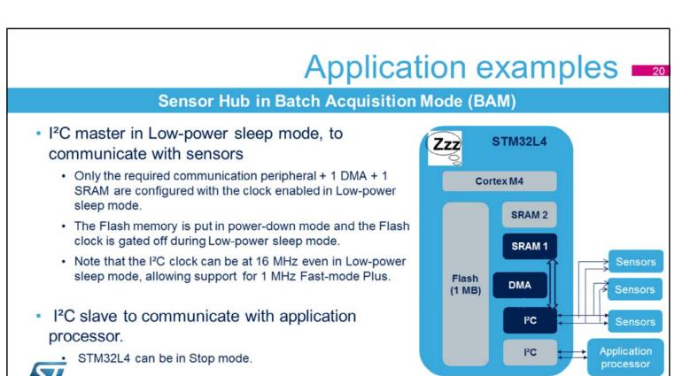
Here is an example of a sensor hub application that requires several I<sup>2</sup>C peripherals.
