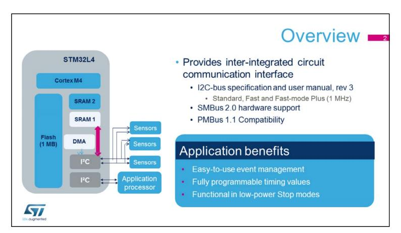
The I<sup>2</sup>C interface is compliant with the NXP I<sup>2</sup>C-bus specification and user manual, Revision 3; the SMBus System Management Bus Specification, Revision 2; and the PMBus Power System Management Protocol Specification, Revision 1.1.
