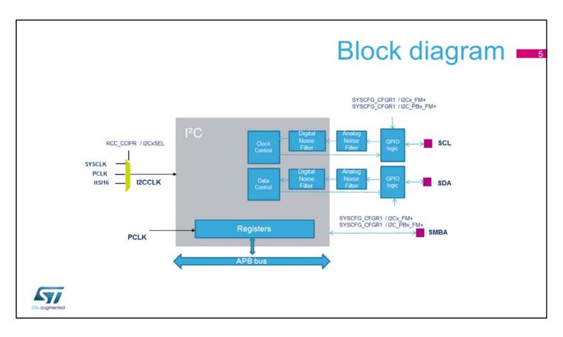
Here is the I<sup>2</sup>C block diagram. The registers are accessed through the APB bus, and the peripheral is clocked with the I<sup>2</sup>C clock, which is independent from the APB clock. The I<sup>2</sup>C clock can be selected between the system clock, APB clock and the high-speed internal 16 MHz RC oscillator.
