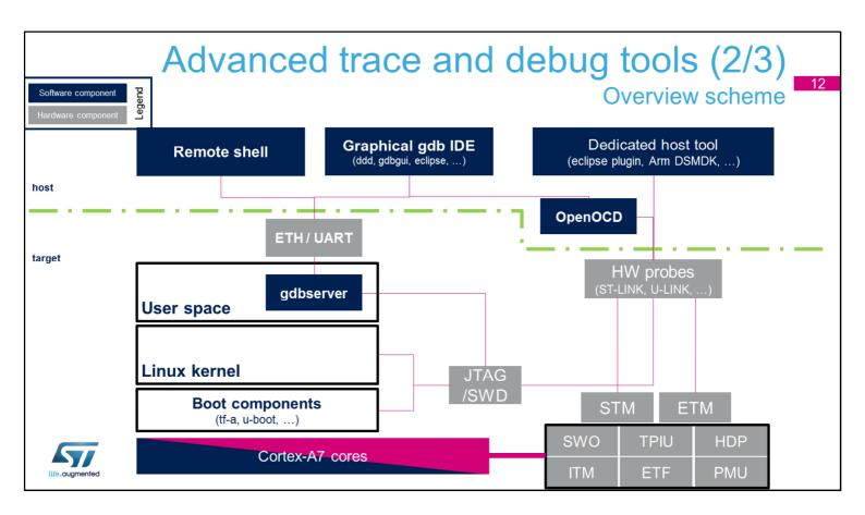
You can find here a representation of the hardware debug configurations detailed in the previous slide.
