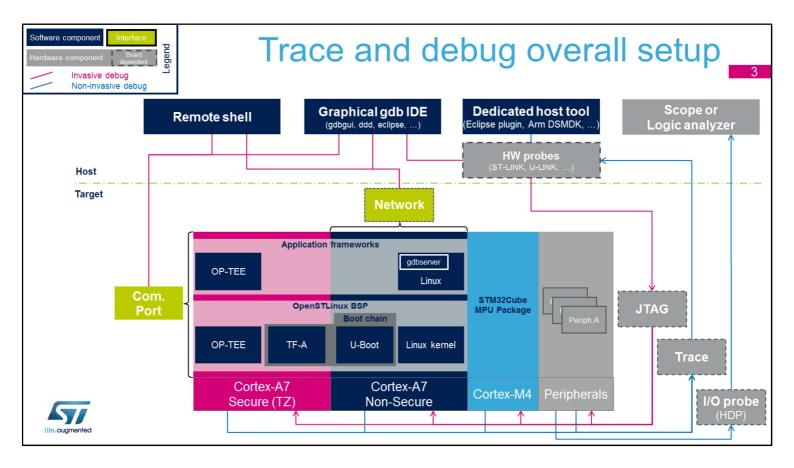
This scheme is a representation of the trace and debug environment on STM32MP1 microprocessors, showing the different hardware and software paths which interface with cores and hardware peripherals on the target side. Host side represents different group of tools to interface with the user, and able to manage and /or display the trace and
