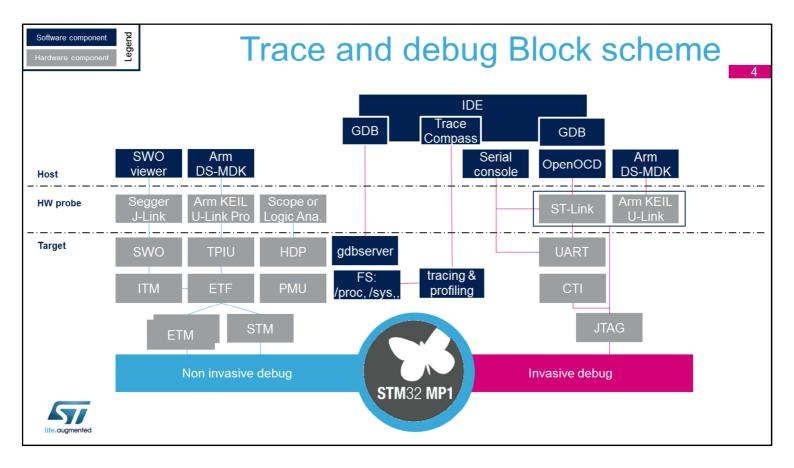
This scheme is a hardware and software block representation, which allows a parallel with the detailed debug block diagram available in the STM32MP1 reference manual. It highlights the main Arm Coresight block IP which is embedded in the STM32MP1 chip.
