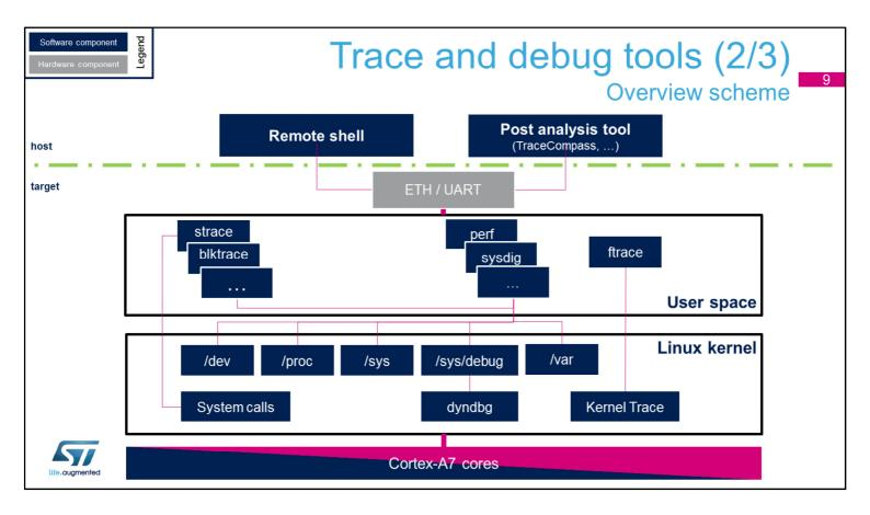
This scheme is a block view representation of the Linux kernel tracing and monitoring links, including some of tools available at user space level.
