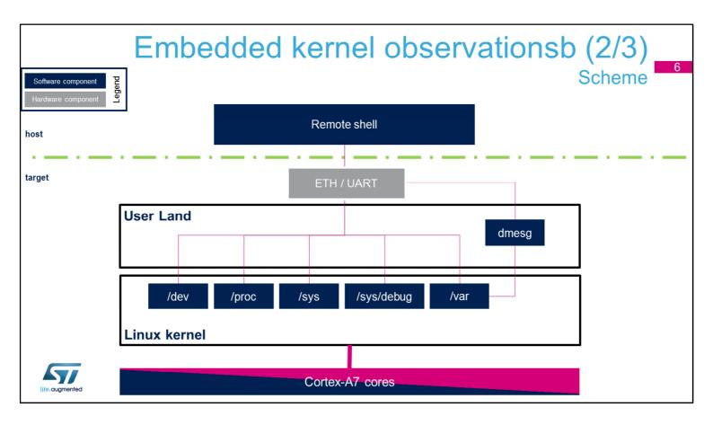
This scheme is an extract from the Trace and debug architecture scheme. It focuses on the Linux kernel observation path and summarizes the information given in the previous slide.
