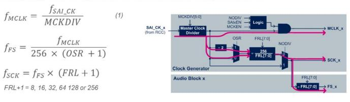
f<sub>MCLK</sub> is the master clock frequency f<sub>B</sub> is the sampling rate frequency (~ frame period) f<sub>SCK</sub> is the bit clock frequency
