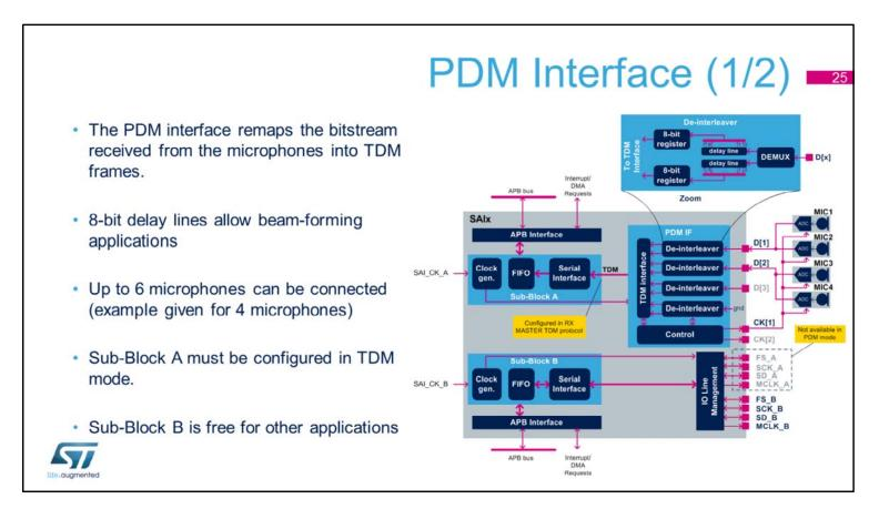
The PDM interface remaps the bitstream received from the digital microphones into TDM frames.
