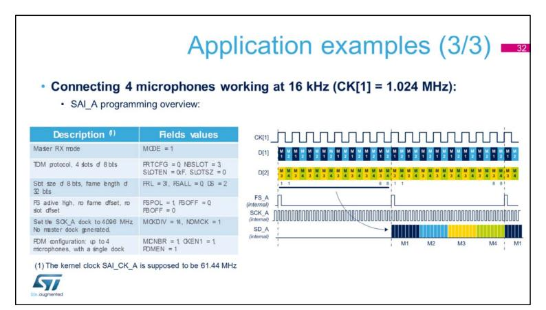
This example shows the most important SAI settings in order to capture the samples provided by 4 digital microphones. In typical applications, the microphones receive a bitstream clock frequency 64 times higher than the wanted audio rate. If the application needs to handle a 16 kHz audio stream, then the bitstream clock provided to the digital microphones must be 16 kHz multiplied by 64, which corresponds to a clock frequency of 1.024 MHz.
