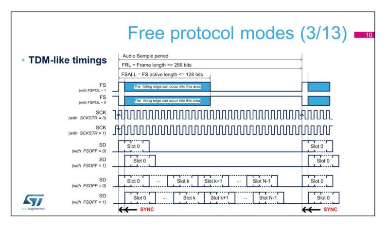
The following example shows some of the possibilities of the interface for the TDM-like protocols. In a TDM-like protocol:
