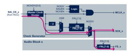
$f_{\text{PS}}$  is the sampling rate frequency (~ frame period)  $f_{\text{SCK}}$  is the bit clock frequency
