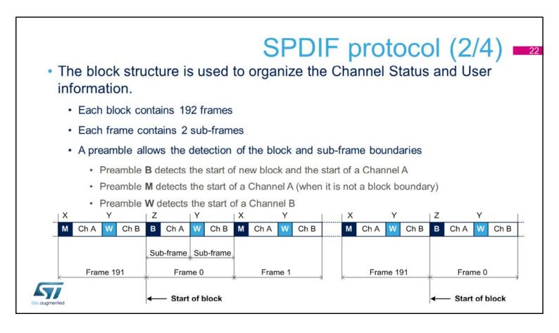
In IEC60958 specifications, the block structure is used to decode the Channel Status (CS), and User information (U).
