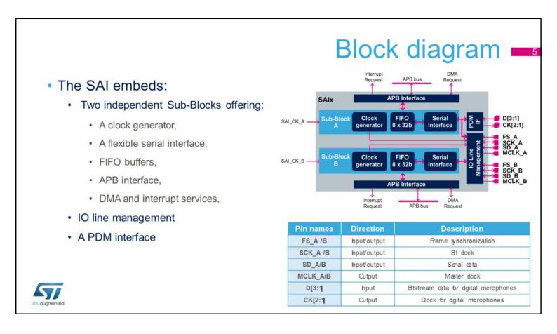
The SAI is composed of two independent sub-blocks (subblock A and B).
