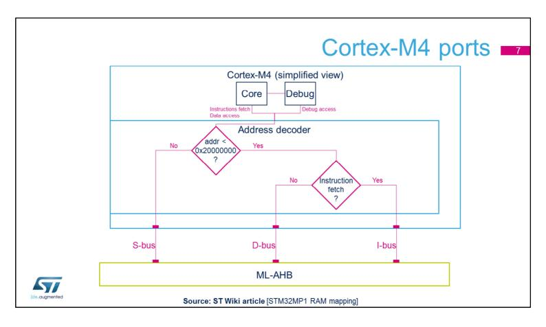
This slide focuses on a Cortex-M4 specificity, since it is connected to the MLAHB interconnect via three different ports, listed below and shown in the figure:
