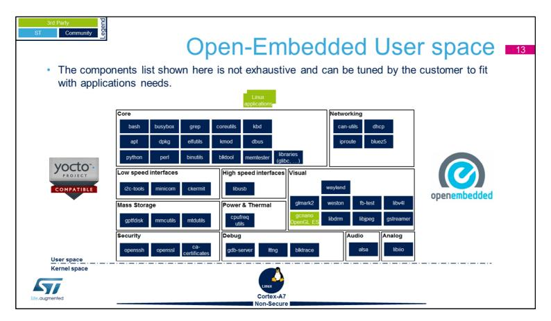
The STM32MPU Embedded Software distribution is build thanks to the Open-Embedded build framework for embedded Linux platforms.
