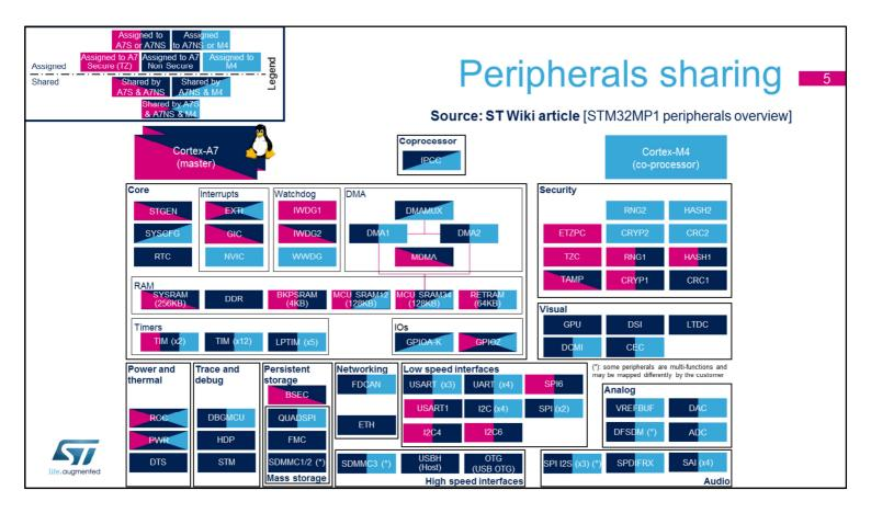
In line with the concepts introduced on the previous slide, the legend of this diagram distinguishes two possible states for each peripheral:
