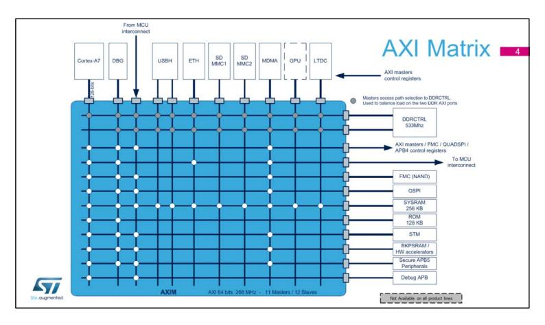
The AXI Matrix is enabling the interconnection between up to 11 masters and 12 slaves peripherals.
