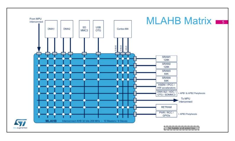
AHB Matrix is enabling the interconnection between up to 10 masters and 9 slaves peripherals.
