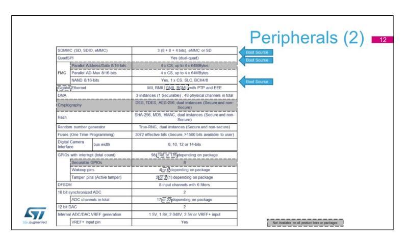
SDMMC can be a boot source by using either SD-Card (SDMMC1) or eMMC (SDMMC2) memory cards. QUADSPI bank1 can be a boot source for Serial-NOR or Serial-NAND Flash memories.
