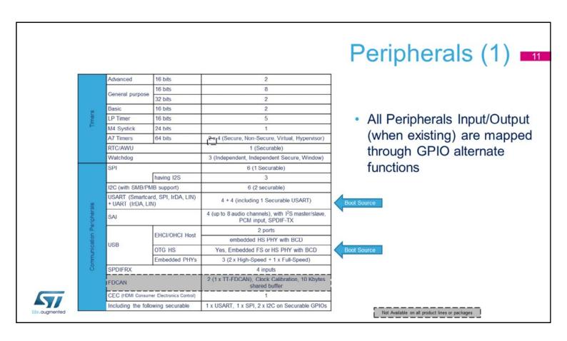
Peripherals with IOs are mapped on GPIO alternate functions (AFMUX).
