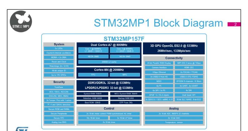
This block diagram summarizes the key features of the STM32MP157F which is part of the high-end line of the STM32MP1 Series.
