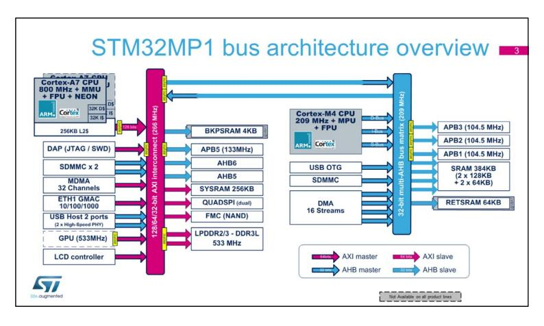
The STM32MP1 bus architecture is split in two interconnect matrix (Arm Cortex-A7 and Arm Cortex-M4) operating in different frequency domains, which can be set in low power modes independently.
