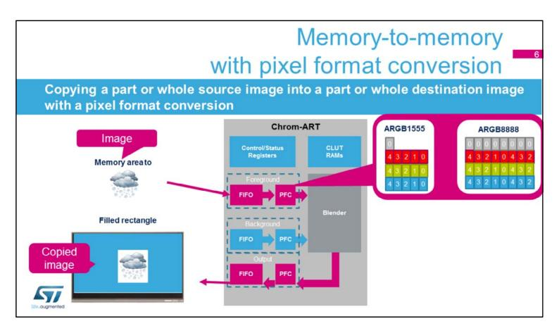
Memory-to-memory mode with pixel format conversion is used to do the same type of copy as Memory-to memory mode but with a pixel format conversion. It can copy an RGB565 image into an RGB888 image without having to use the CPU.
