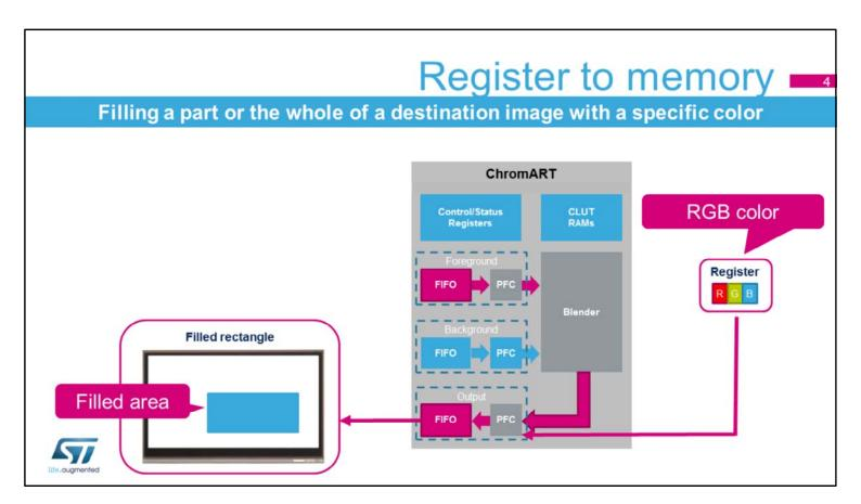
Register-to-memory mode is used to fill a part or whole destination image with a specific color.
