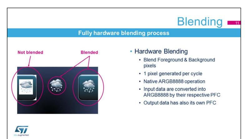
The fully hardware blender allows to blend a foreground image and a background image with transparency.
