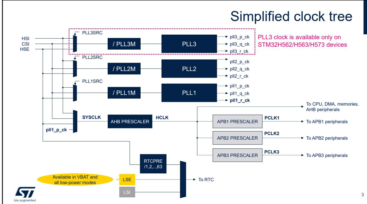
The system clock can be derived from the high-speed internal 64 MHz RC oscillator (HSI), from the high-speed external 4 to 50 MHz oscillator (HSE), from the low-power oscillator (CSI) or from the pll1\_p\_ck output of the PLL1. The AHB clock, called HCLK, is derived by dividing the system clock by a programmable prescaler.
