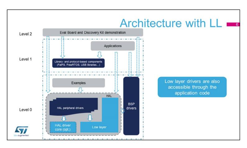
The STM32L4 firmware architecture allows applications to directly access HAL peripheral drivers or low layer drivers without using HAL peripheral drivers.
