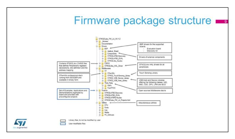
The STM32CubeL4 firmware solution comes in a single ZIP file having the structure shown in this slide for all STM32 series.
