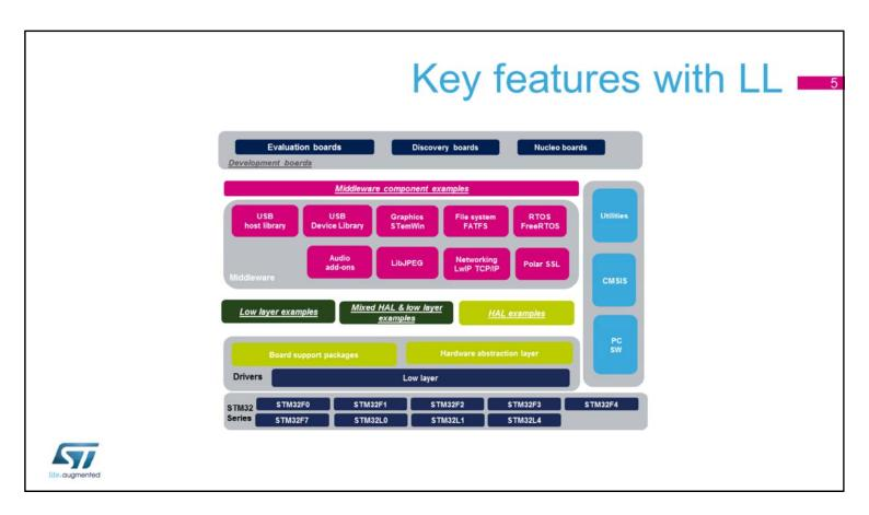
Low layer drivers are included in the STM32CubeL4 package along with some examples using either the HAL, low layer drivers or both.
