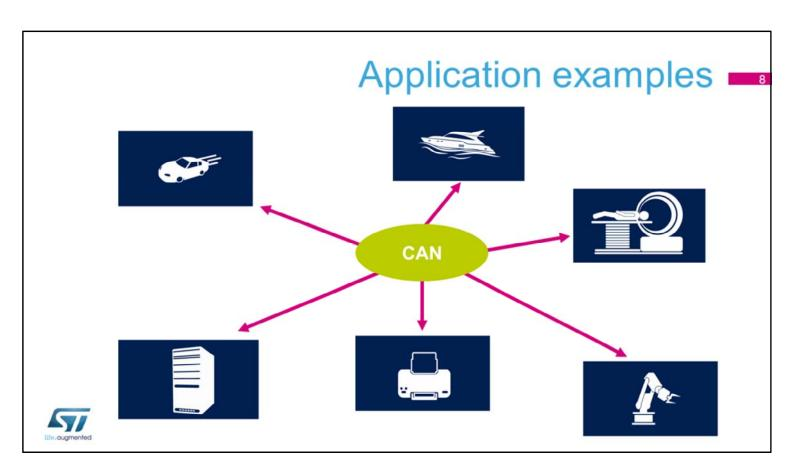
The controller area network (CAN bus) was originally designed for automotive applications, but is now also used in many other contexts.
