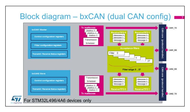
This simplified block diagram of the BxCAN in dual CAN configuration shows the shared 28 Acceptance filters between the two BxCAN modules.
