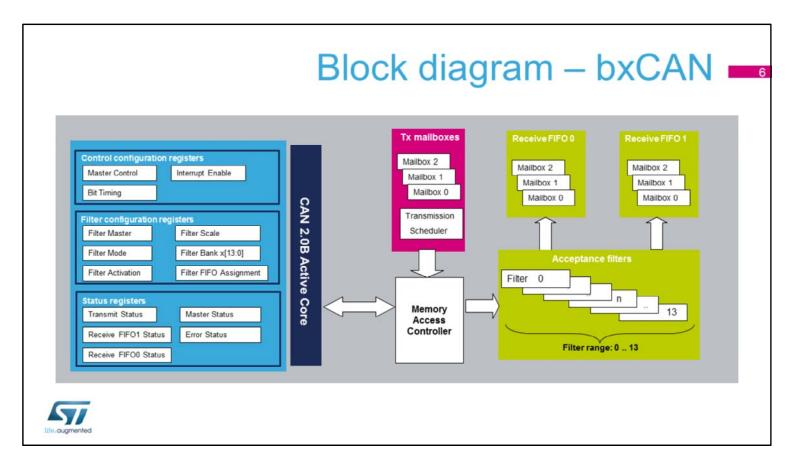
This simplified block diagram of the CAN shows its basic functional and control features.
