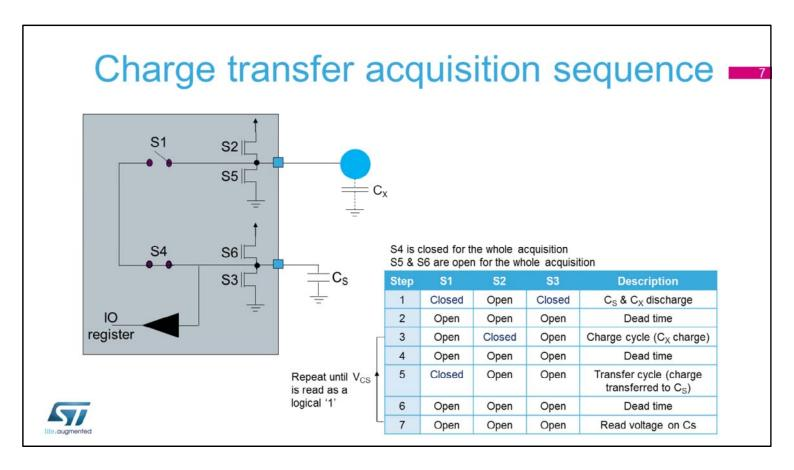
The charge transfer acquisition sequence is composed of 7 steps.
