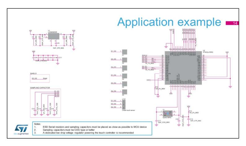
This example details a solution with 6 touchkeys and one linear touch sensor. It is important to note that a dedicated voltage regulator is used and that the solution also uses the active shield for optimum conducted noise robustness. A COG type capacitor is used for the sampling capacitors as they offer a good stability over the temperature range and no memory effect.
