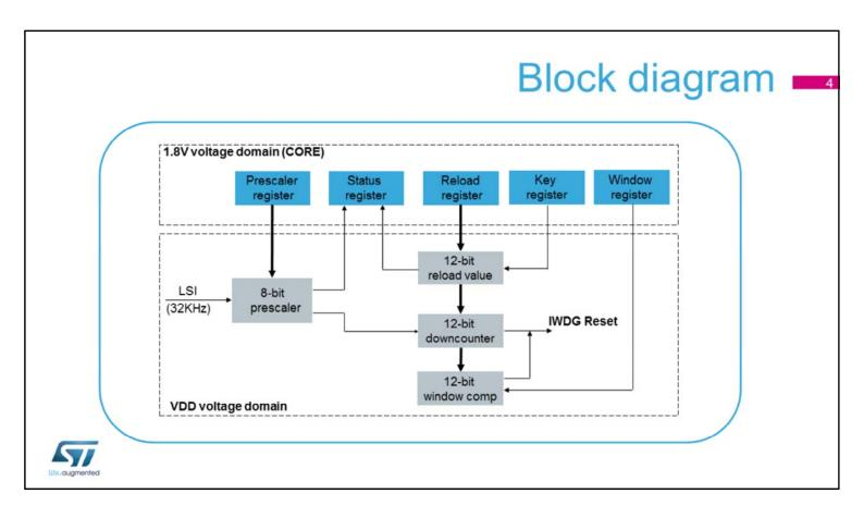
The IWDG registers are located in the CORE voltage domain while its functions are in the VDD voltage domain. This architecture makes it possible for the IWDG to continue operating in Stop and Standby modes. The 8-bit prescaler is used to divide the LSI oscillator frequency.
