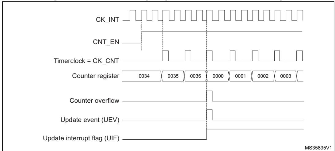
**Figure 208. Counter timing diagram, internal clock divided by 4**
