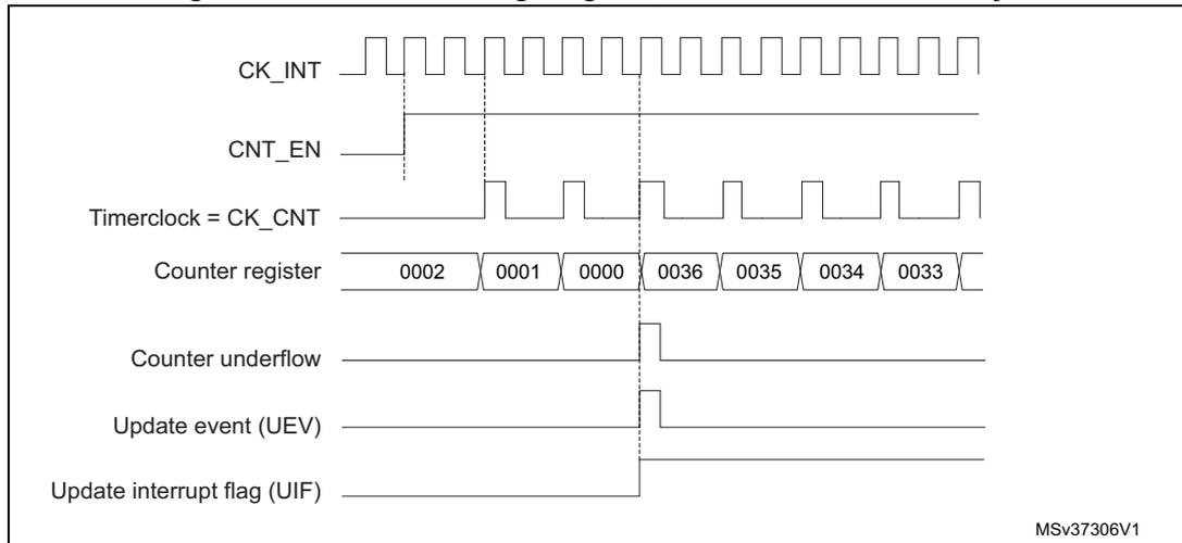
**Figure 145. Counter timing diagram, internal clock divided by 4**
