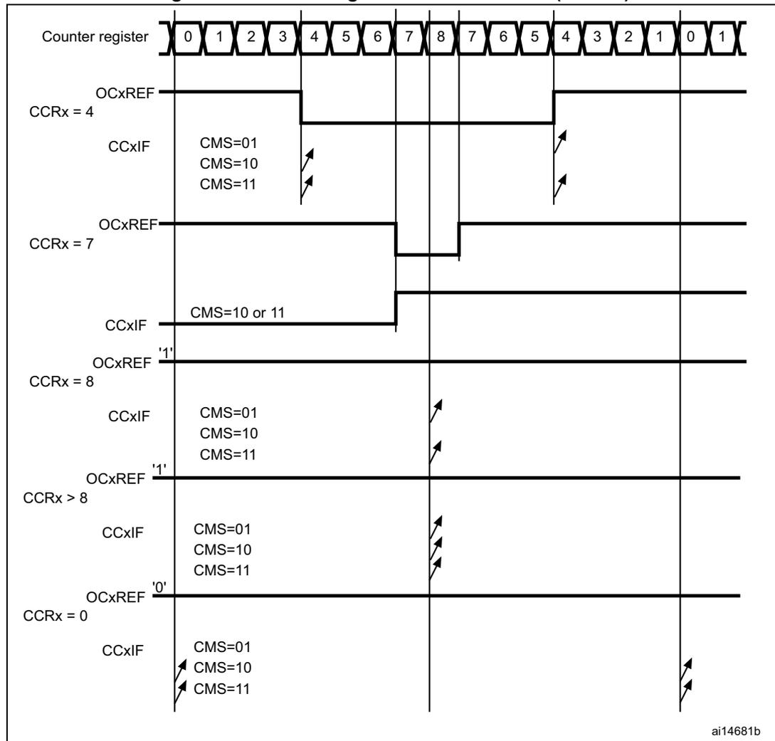
Hints on using center-aligned mode:
