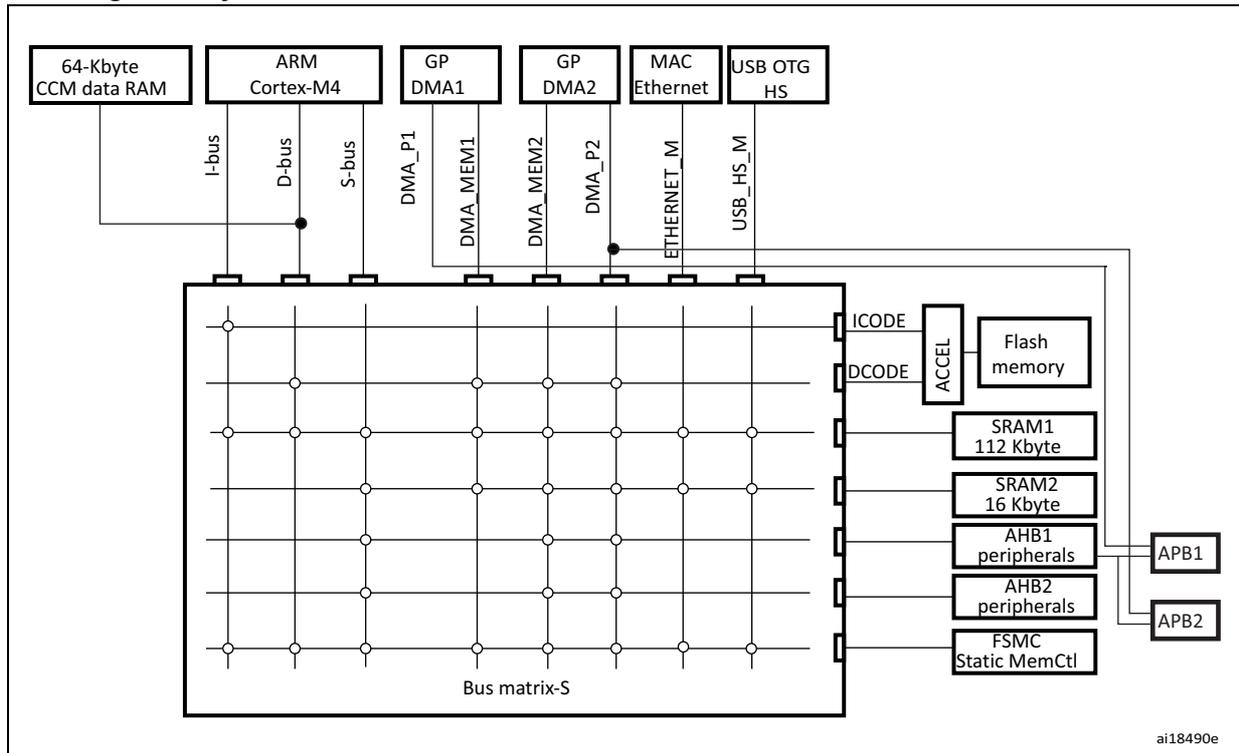
In the STM32F42xx and STM32F43xx devices, the main system consists of 32-bit multilayer AHB bus matrix that interconnects:
