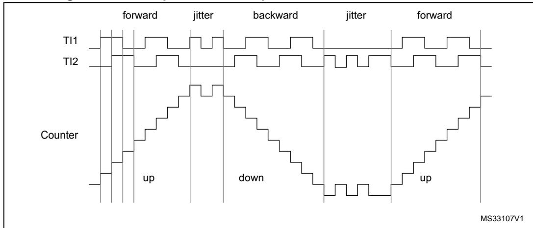
Figure 128 gives an example of counter behavior when TI1FP1 polarity is inverted (same configuration as above except CC1P='1').
