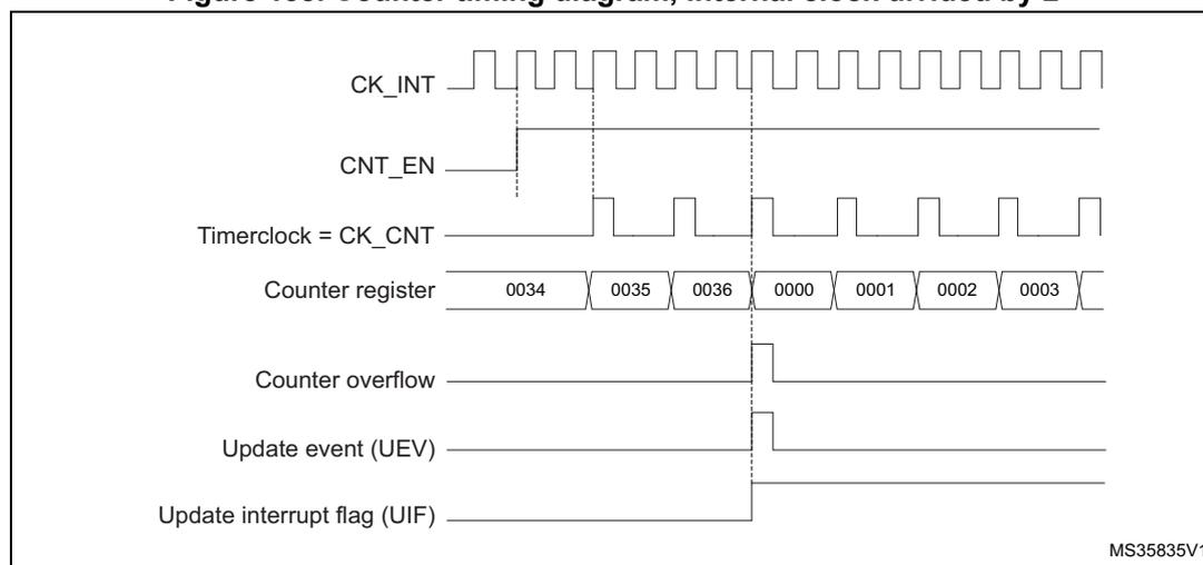
**Figure 139. Counter timing diagram, internal clock divided by 4**
