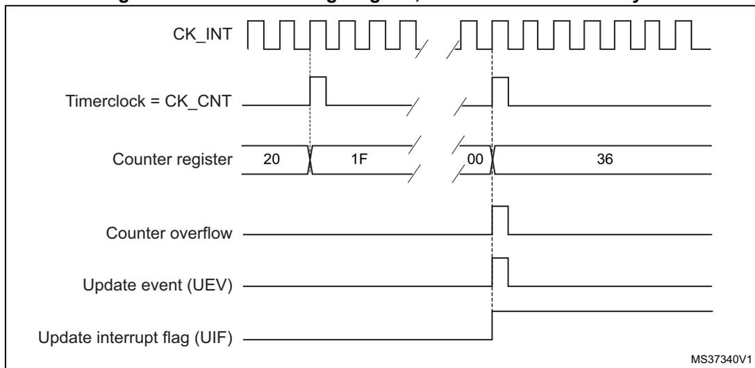
Figure 147. Counter timing diagram, Update event
