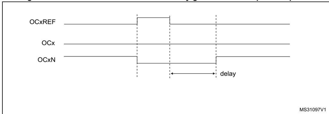
The dead-time delay is the same for each of the channels and is programmable with the DTG bits in the TIMx\_BDTR register. Refer to [Section 17.4.18: TIM1 and TIM8 break and dead-time register \(TIMx\\_BDTR\)](#) for delay calculation.
