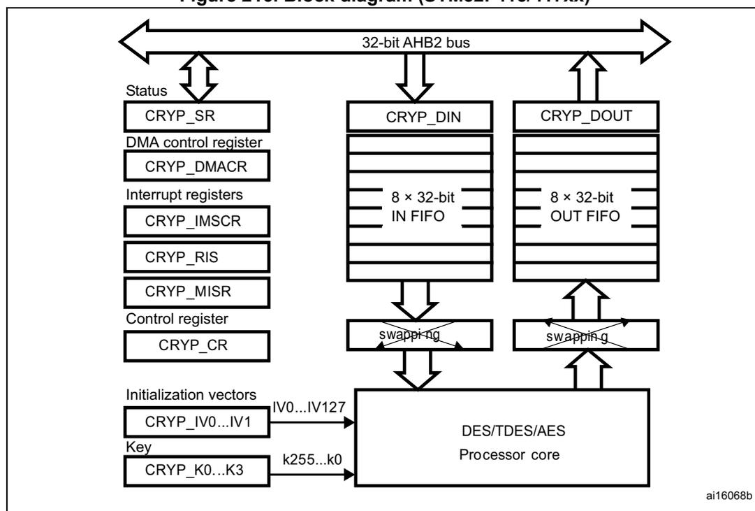
Figure 217. Block diagram (STM32F43xxx)
