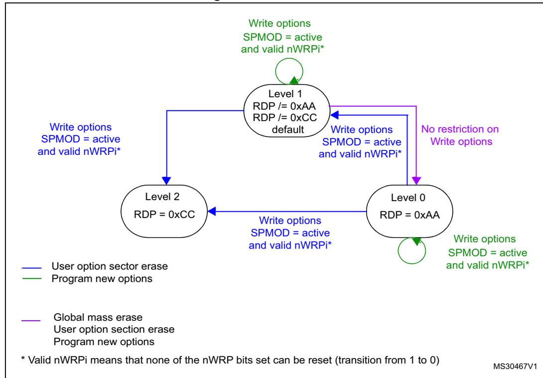
The deactivation of the SPRMOD and/or the unprotection of PCROPed user sectors can only occur when, at the same time, the RDP level changes from 1 to 0. If this condition is not respected, the user option byte modification is cancelled and the write error WRPERR flag is set. The modification of the users option bytes (BOR\_LEV, RST\_STDBY, ..) is allowed since none of the active nWRPi bits is reset and SPRMOD is kept active.
