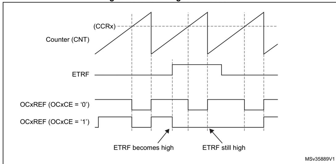
*Note:* In case of a PWM with a 100% duty cycle (if CCR<sub>x</sub>>ARR), then OCxREF is enabled again at the next counter overflow.
