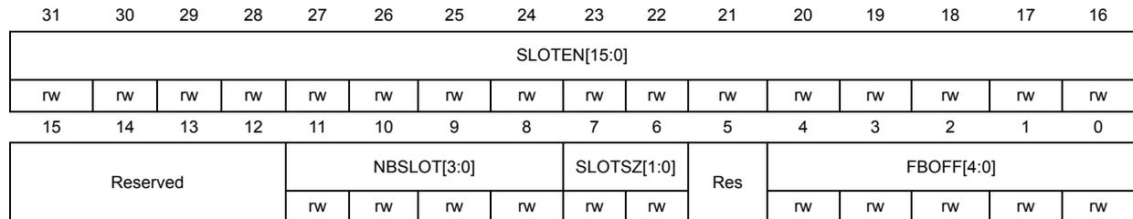
Bits 31:16 **SLOTEN[15:0]**: Slot enable. These bits are set and cleared by software.
