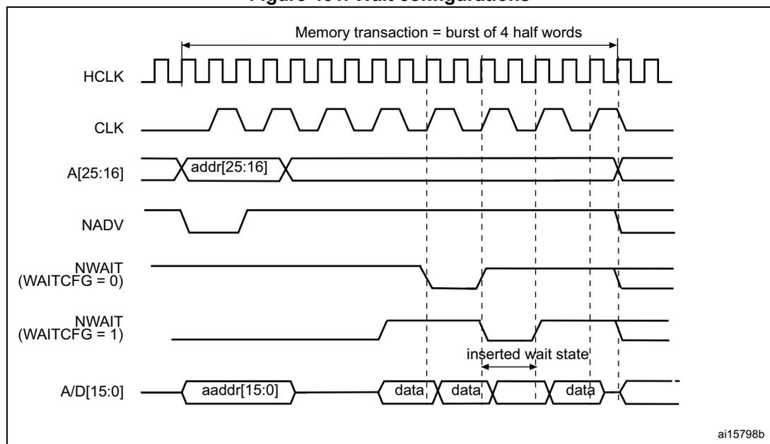
Figure 452. Synchronous multiplexed read mode - NOR, PSRAM (CRAM)
