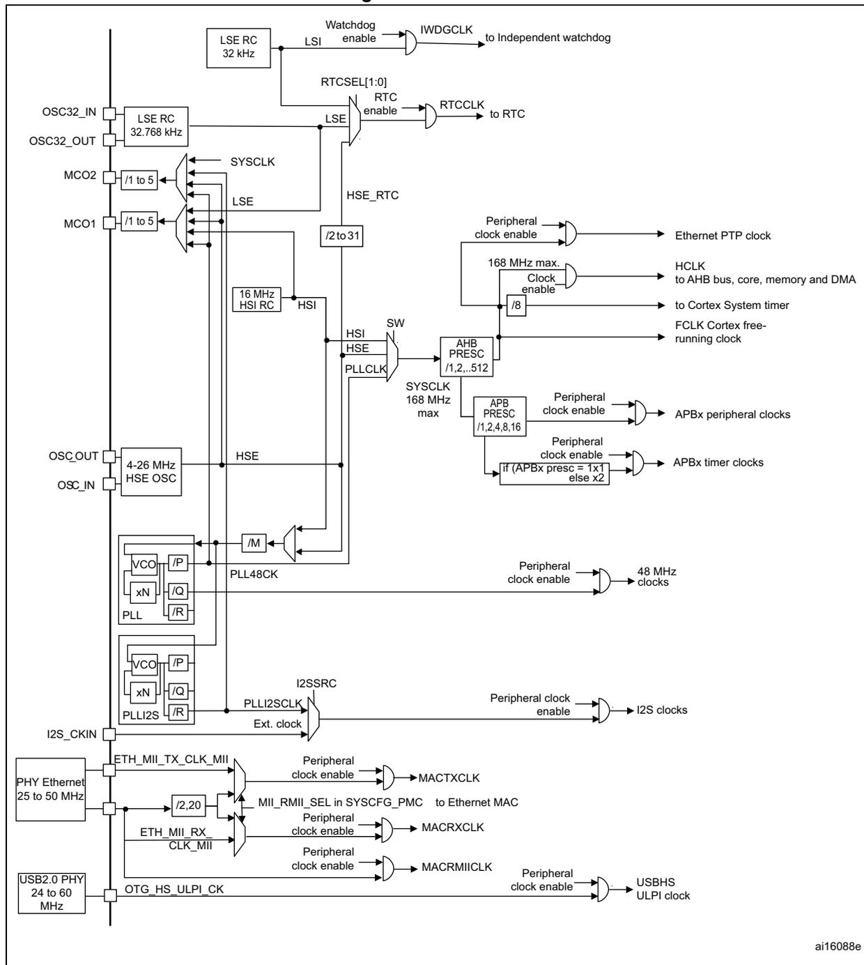
1. For full details about the internal and external clock source characteristics, refer to the Electrical characteristics section in the device datasheet.
