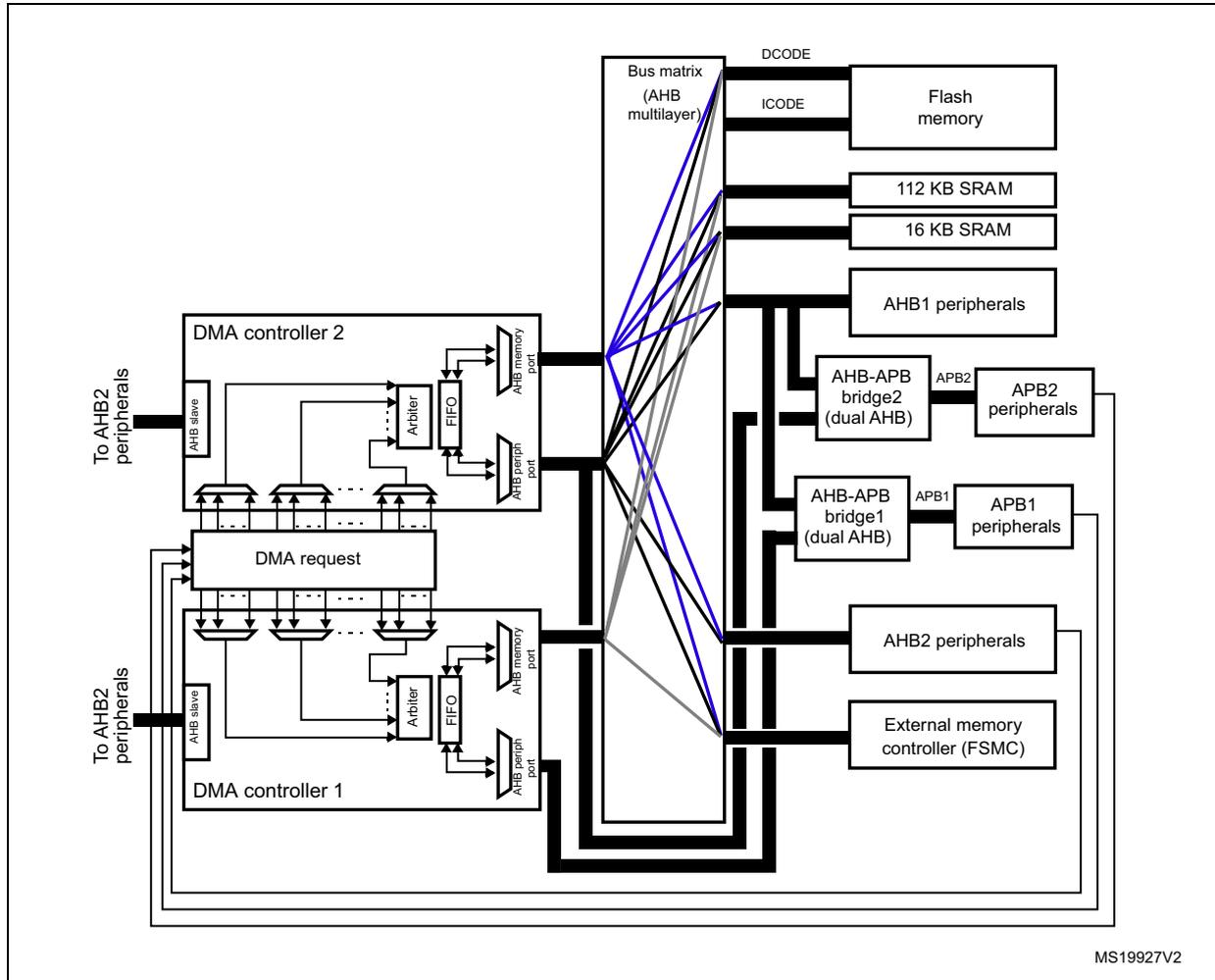
1. The DMA1 controller AHB peripheral port is not connected to the bus matrix like DMA2 controller. As a result, only DMA2 streams are able to perform memory-to-memory transfers.
