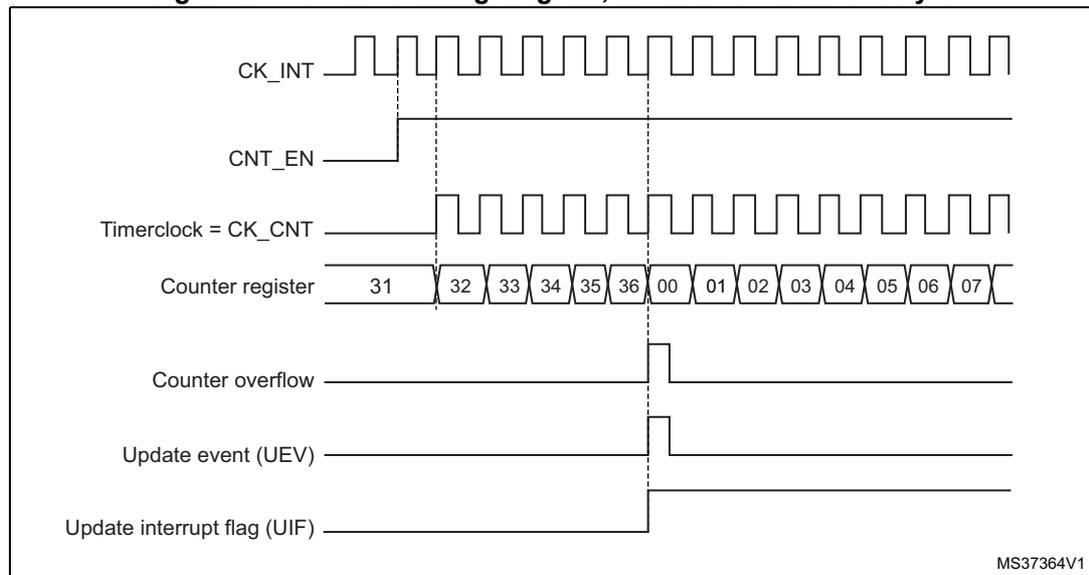
**Figure 207. Counter timing diagram, internal clock divided by 2**
