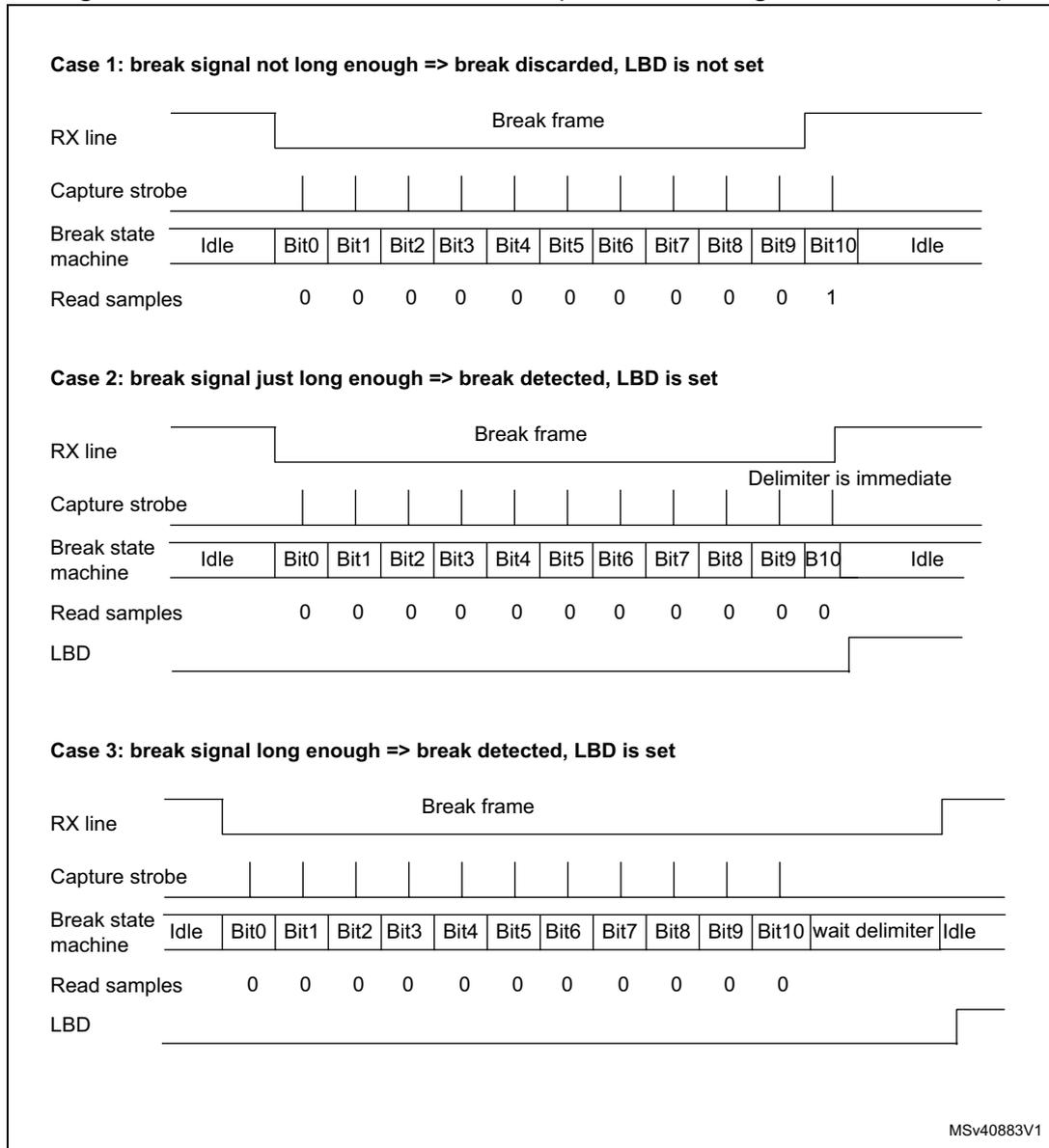
Figure 306. Break detection in LIN mode vs. Framing error detection
