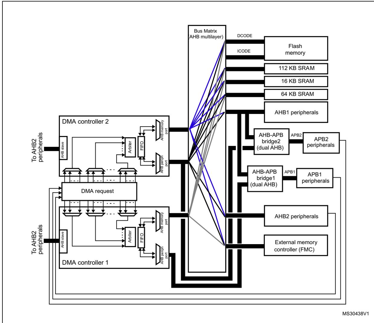
1. The DMA1 controller AHB peripheral port is not connected to the bus matrix like in the case of the DMA2 controller, thus only DMA2 streams are able to perform memory-to-memory transfers.
