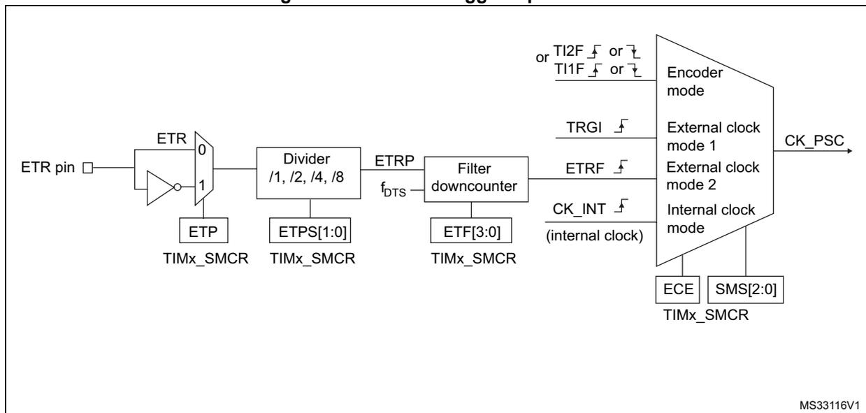
For example, to configure the upcounter to count each 2 rising edges on ETR, use the following procedure:
