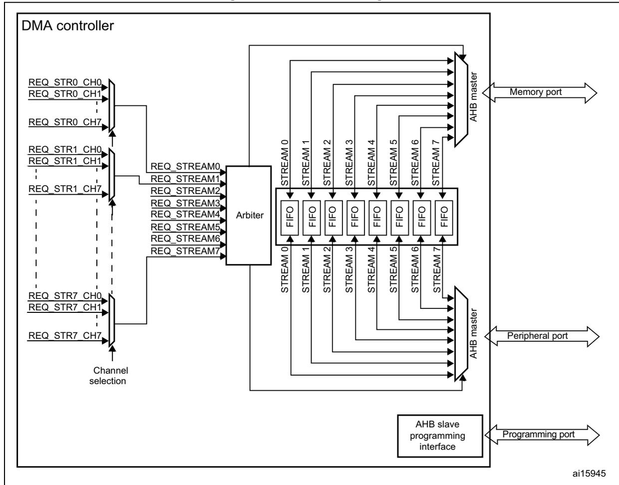
The DMA controller performs direct memory transfer: as an AHB master, it can take the control of the AHB bus matrix to initiate AHB transactions.
