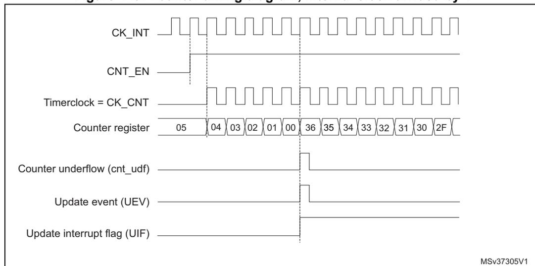
**Figure 144. Counter timing diagram, internal clock divided by 2**
