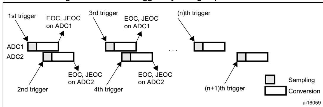
If the injected discontinuous mode is enabled for both ADC1 and ADC2:
