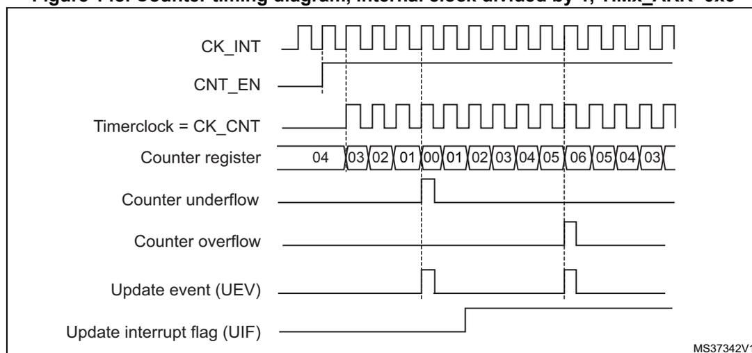
1. Here, center-aligned mode 1 is used, for more details refer to [Section 18.4.1: TIMx control register 1 \(TIMx\\_CR1\)](#).
