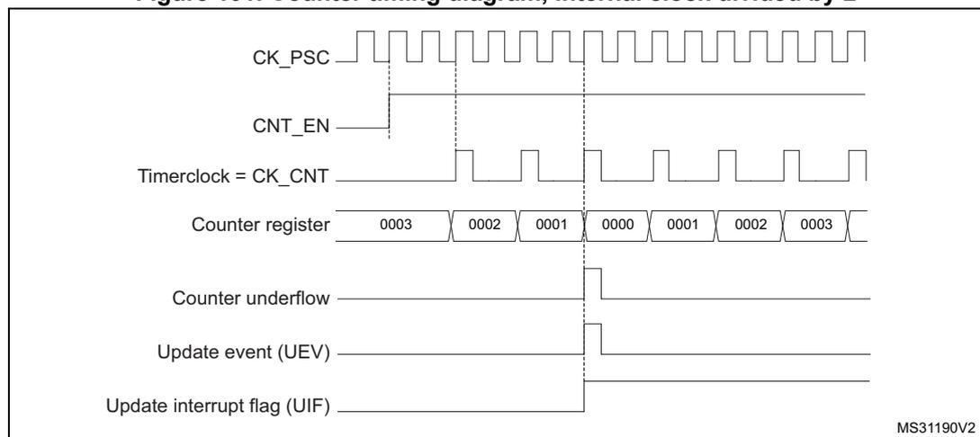
**Figure 102. Counter timing diagram, internal clock divided by 4, TIMx\_ARR=0x36**
