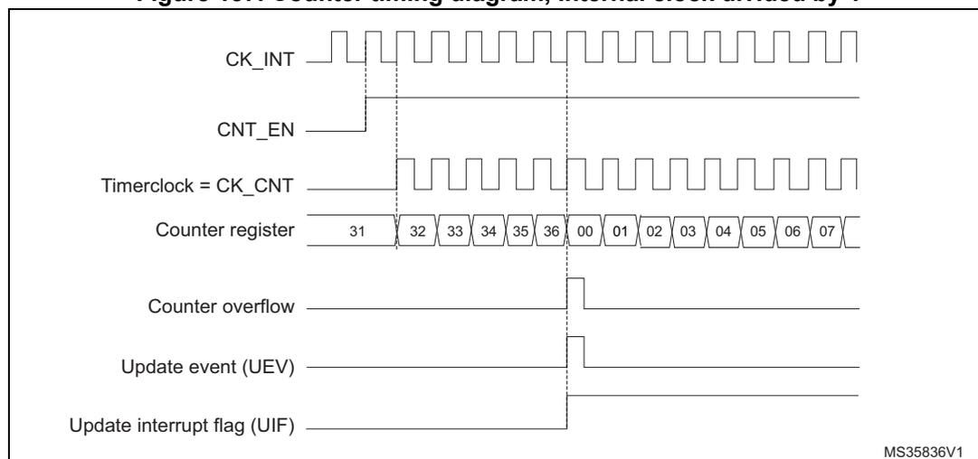
**Figure 138. Counter timing diagram, internal clock divided by 2**
