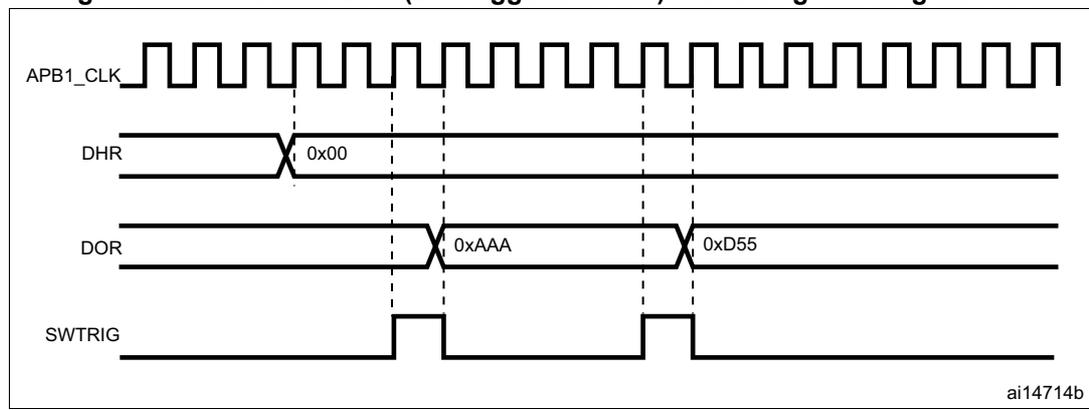
*Note:* The DAC trigger must be enabled for noise generation by setting the TEN<sub>x</sub> bit in the DAC\_CR register.
