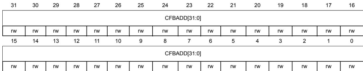
Bits 31:0 **CFBADD[31:0]**: Color Frame Buffer Start Address
