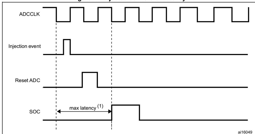
1. The maximum latency value can be found in the electrical characteristics of the STM32F40x and STM32F41x datasheets.
