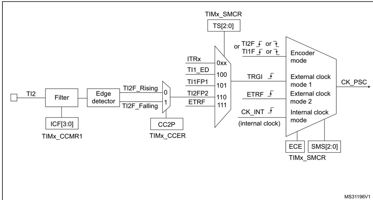
For example, to configure the upcounter to count in response to a rising edge on the TI2 input, use the following procedure:
