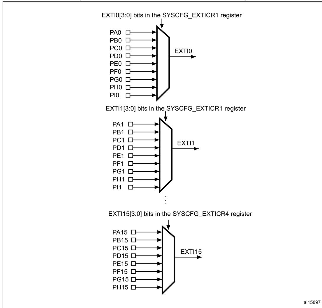
Figure 43. External interrupt/event GPIO mapping (STM32F42xxx and STM32F43xxx)
