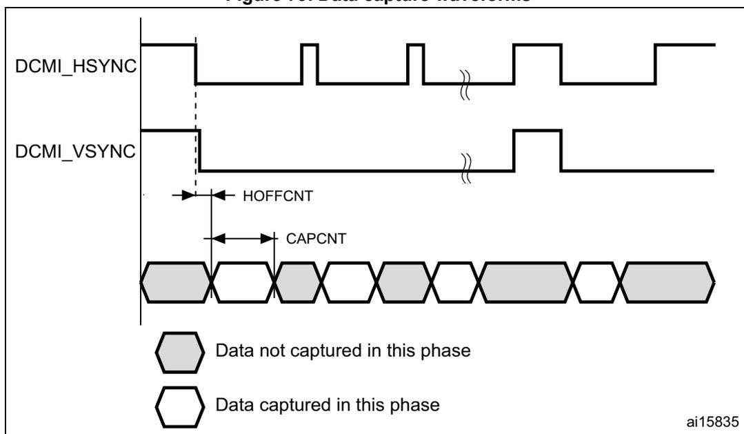
1. Here, the active state of DCMI\_HSYNC and DCMI\_VSYNC is 1.
