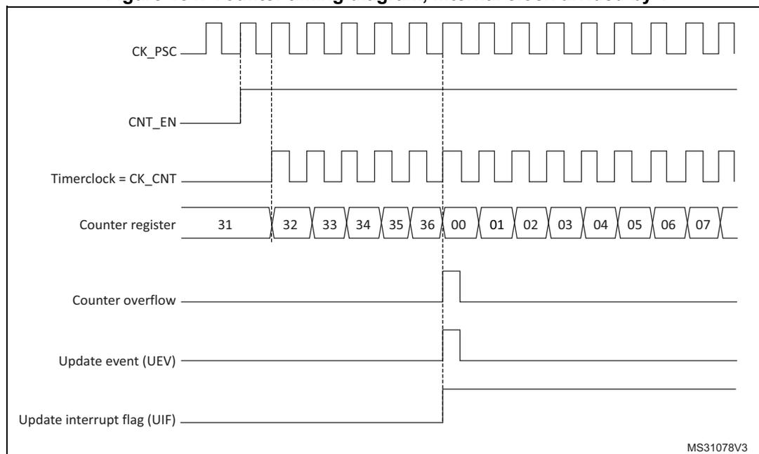
**Figure 185. Counter timing diagram, internal clock divided by 2**
