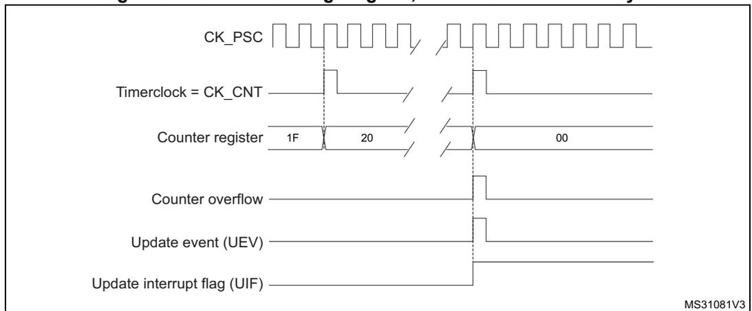
**Figure 188. Counter timing diagram, update event when ARPE=0 (TIMx\_ARR not preloaded)**
