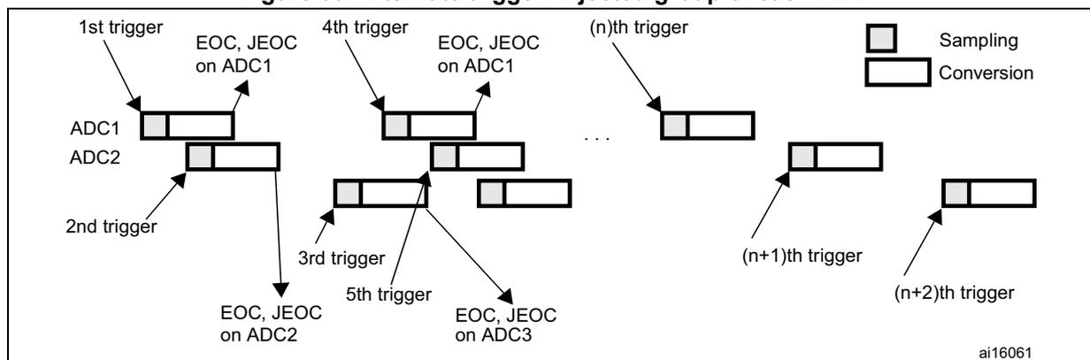
**13.9.5 Combined regular/injected simultaneous mode**
