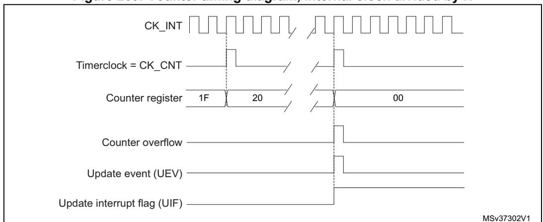
**Figure 210. Counter timing diagram, update event when ARPE=0 (TIMx\_ARR not preloaded)**
