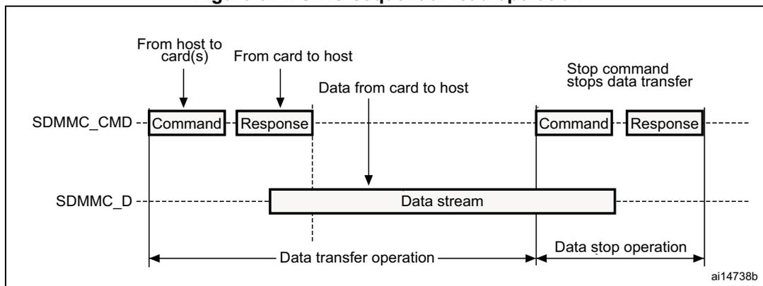
Figure 325. SDIO sequential write operation
