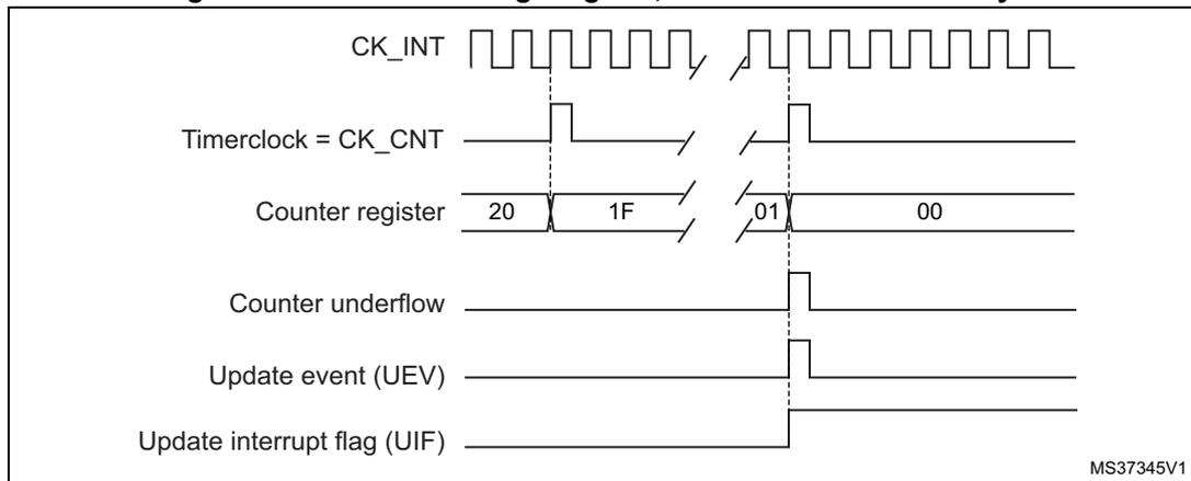
**Figure 152. Counter timing diagram, Update event with ARPE=1 (counter underflow)**
