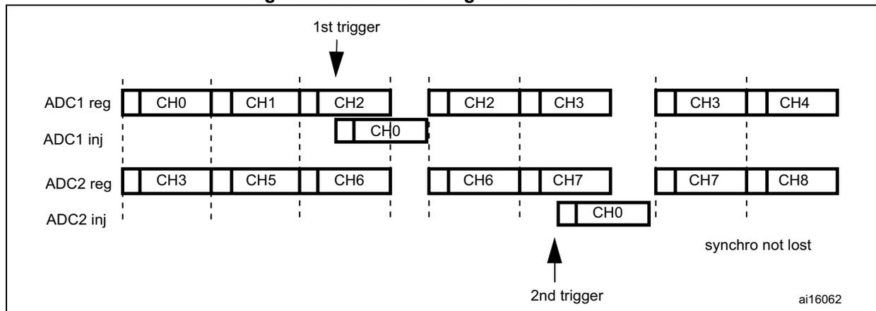
If a trigger occurs during an injected conversion that has interrupted a regular conversion, it is ignored. *Figure 62* shows the behavior in this case (2nd trigger is ignored).
