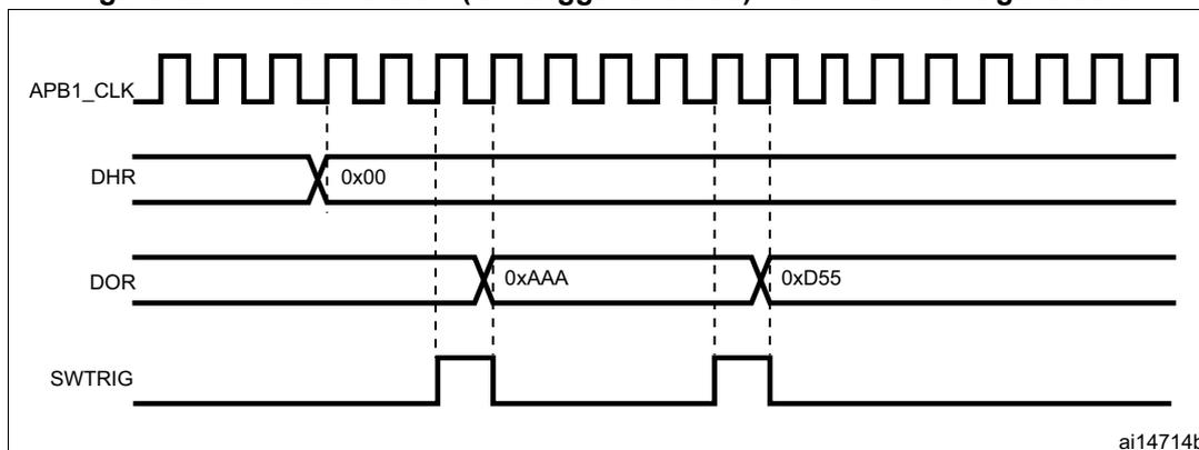
Note: The DAC trigger must be enabled for noise generation by setting the TENx bit in the DAC\_CR register.
