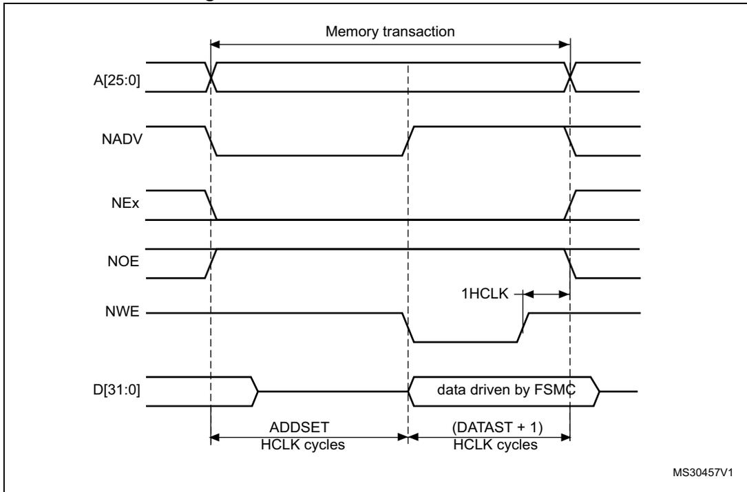
Figure 464. ModeB write access waveforms
