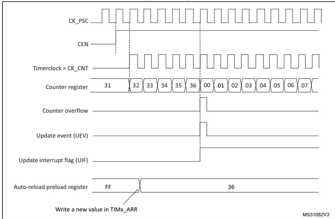
**Figure 189. Counter timing diagram, update event when ARPE=1 (TIMx\_ARR preloaded)**
