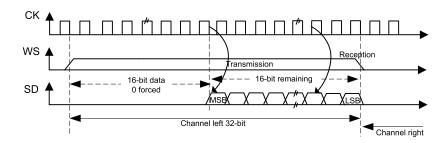
When 16-bit data frame extended to 32-bit channel frame is selected during the I<sup>2</sup>S configuration phase. Only one access to the SPIx\_DR register is required. The 16 remaining bits are forced by hardware to 0x0000 to extend the data to 32-bit format. In this case it corresponds to the half-word MSB.
