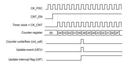
Figure 38. Counter timing diagram, internal clock divided by 2
