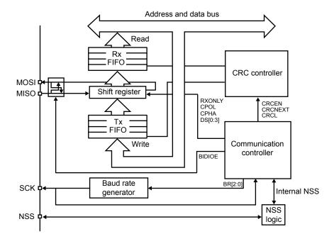
Figure 150. SPI block diagram
