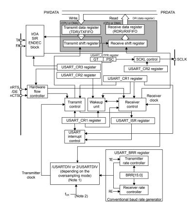
Figure 113. USART block diagram
