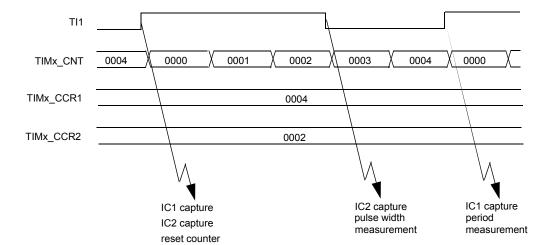
Figure 60. PWM input mode timing
