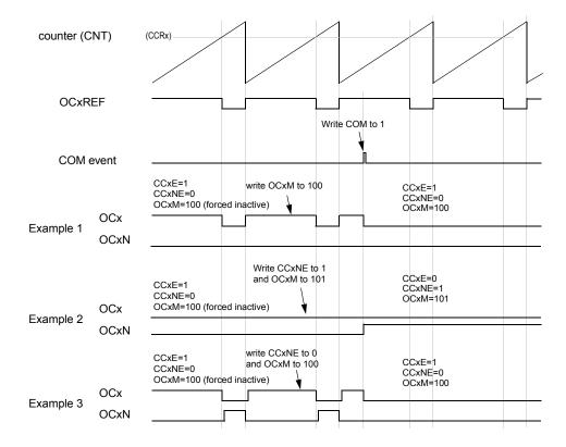
Figure 75. 6-step generation, COM example (OSSR=1)
