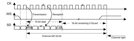
When 16-bit data frame extended to 32-bit channel frame is selected during the I<sup>2</sup>S configuration phase, only one access to the SPIx\_DR register is required. The 16 remaining bits are forced by hardware to 0x0000 to extend the data to 32-bit format.
