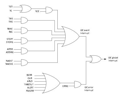
Figure 112. I<sup>2</sup>C interrupt mapping diagram
