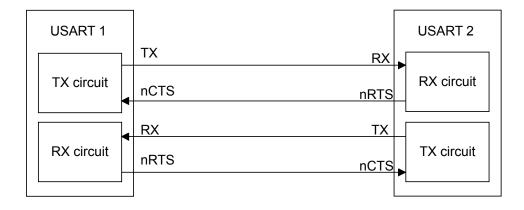
RS232 RTS and CTS flow control can be enabled independently by writing the RTSE and CTSE bits respectively to 1 (in the USART\_CR3 register).
