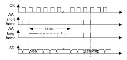
Figure 181. PCM standard waveforms (16-bit)
