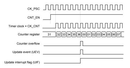
Figure 32. Counter timing diagram, internal clock divided by 2
