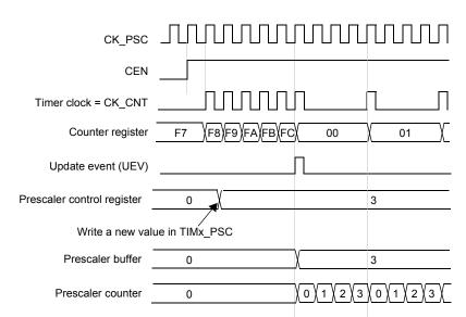
Figure 30. Counter timing diagram with prescaler division change from 1 to 4
