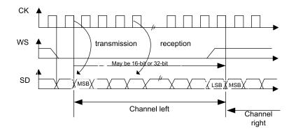
Figure 166. I<sup>2</sup>S Philips protocol waveforms (16/32-bit full accuracy, CPOL = 0)
