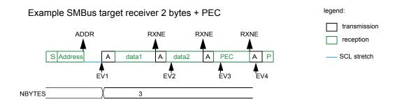
EV1: ADDR ISR: check ADDCODE and DIR, program NBYTES = 3, PECBYTE=1, RELOAD=0, set ADDRCF
