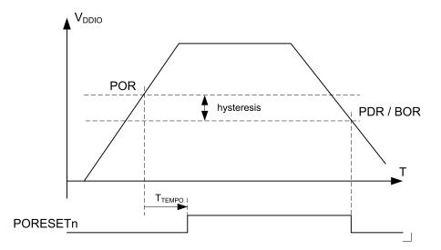
Figure 5. Power-on reset/power-down reset waveform
