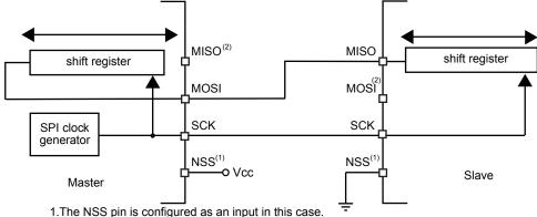
Figure 152. Half-duplex single master/single slave application
