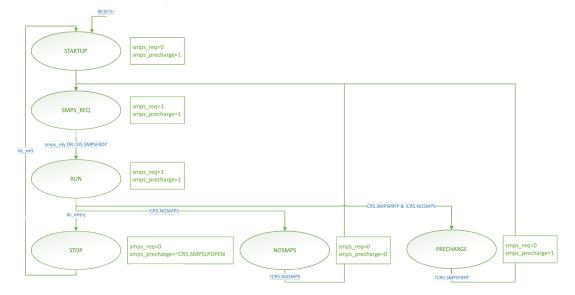
Figure 11. PWRC SMPS state machine overview
