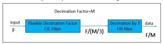
Table 32. Output data rate with ADC input at 1 MHz for analog mode and Table 33. CIC filter output frequency with digital microphone input list the decimation factors and the output frequencies according to the supported inputs (ADC or digital microphone).
