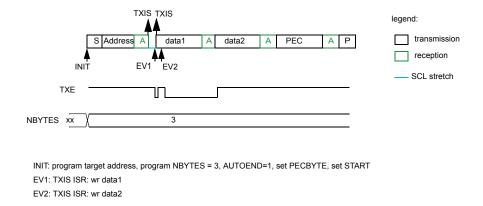
Example SMBus controller transmitter 2 bytes + PEC, software end mode (RESTART)
