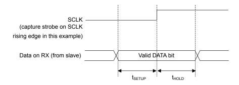
$t_{\text{SETUP}} = t_{\text{HOLD}} \ 1/16 \ \text{bit time}$
