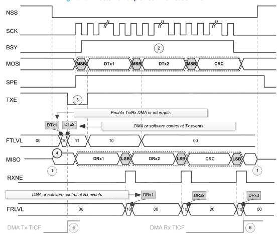
Figure 161. Master full-duplex communication with CRC
