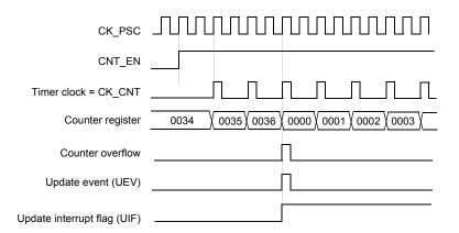
Figure 33. Counter timing diagram, internal clock divided by 4
