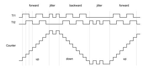
Figure 79. Example of encoder interface mode with TI1FP1 polarity inverted gives an example of counter behavior when TI1FP1 polarity is inverted (same configuration as above except CC1P='1').
