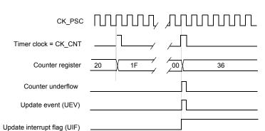
Figure 40. Counter timing diagram, internal clock divided by N
