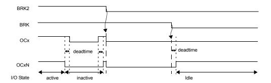
Figure 73. PWM output state following BRK assertion (OSSI=0)
