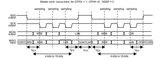
Note: Similar behavior is encountered when CPOL=0. In this case the sampling edge is the rising edge of SCK, and NSS assertion and de-assertion refer to this sampling edge.
