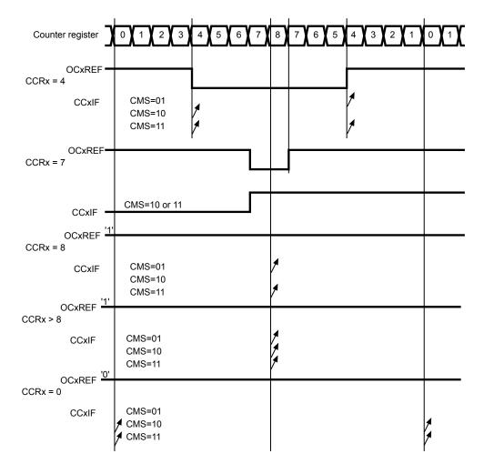
Figure 63. Center-aligned PWM waveforms (ARR=8)
