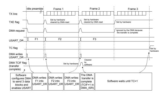
Figure 133. Transmission using DMA
