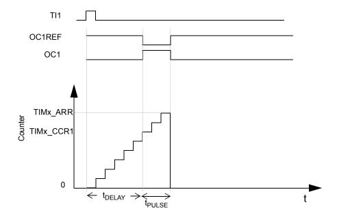
Figure 76. Example of one-pulse mode
