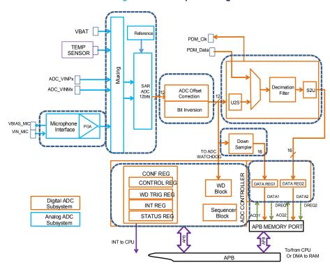
Figure 22. ADC top level diagram
