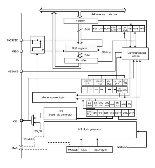
Figure 165. I<sup>2</sup>S block diagram
