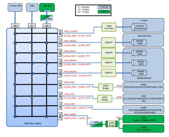
Figure 1. STM32WB07xC and STM32WB06xC system architecture
