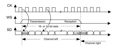
Figure 175. LSB justified 16-bit or 32-bit full-accuracy length with CPOL = 0
