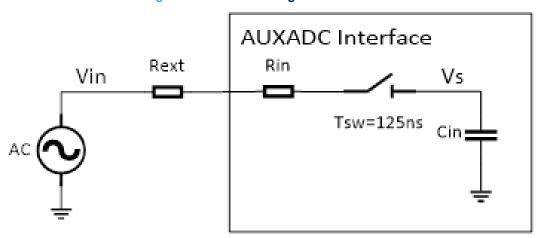
Knowing that: Rin=550  $\Omega$ , Cin=4 pF, and imposing a maximum sampling error of 1/2 bits, we can determine the maximum input resistance as below:
