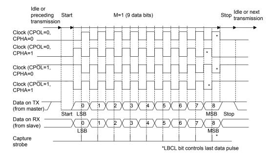
Figure 127. USART data clock timing diagram (M bits = 01)
