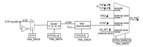
For example, to configure the upcounter to count each 2 rising edges on ETR, use the following procedure:
