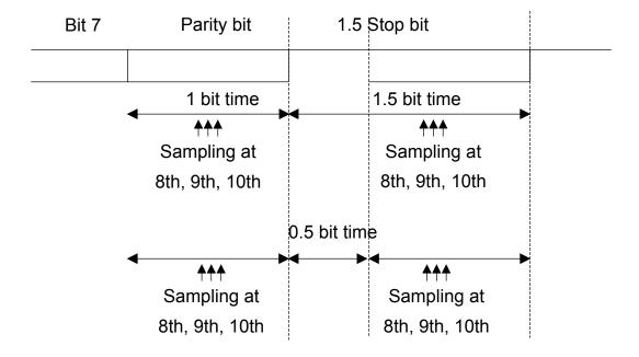
Figure 130. Parity error detection using 1.5 stop bits
