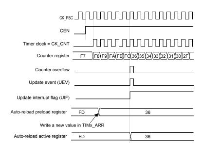
Figure 47. Counter timing diagram, update event with ARPE=1 (counter overflow)
