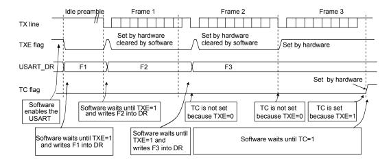
Figure 116. TC/TXE behavior when transmitting
