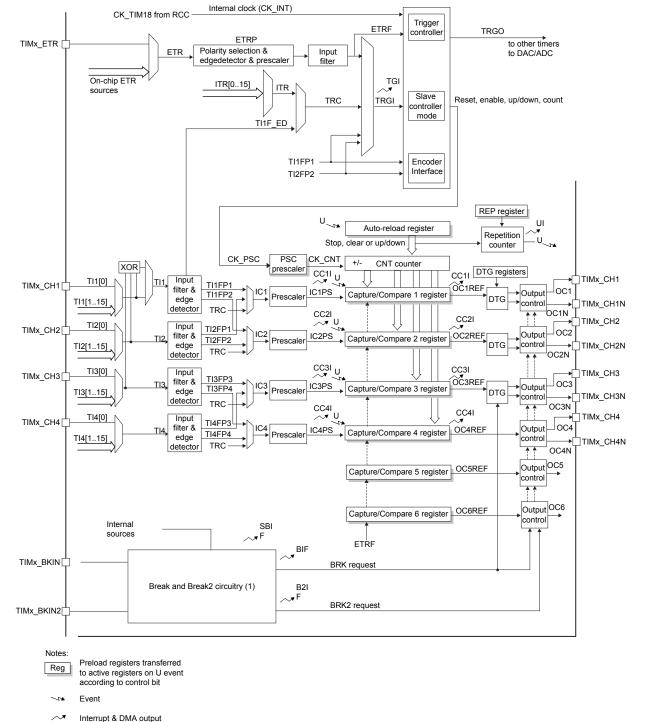
Figure 28. Advanced-control timer block diagram
