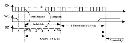
Figure 167. I<sup>2</sup>S Philips standard waveforms (24-bit frame with CPOL = 0)
