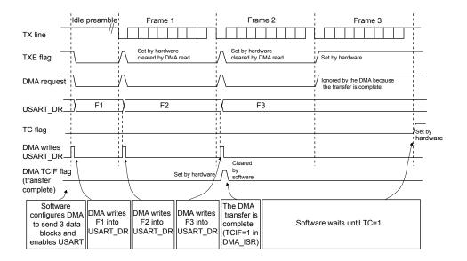
Figure 145. Transmission using DMA
