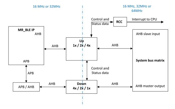
Figure 3. AHB up/down converter
