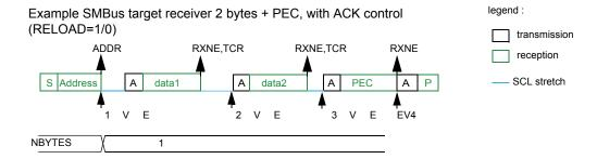
EV1: ADDR ISR: check ADDCODE and DIR, programNBYTES = 1, PECBYTE=1, RELOAD=1, set ADDRCF
