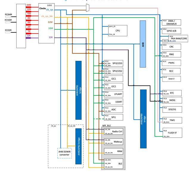
Figure 13. Peripheral clock tree overview
