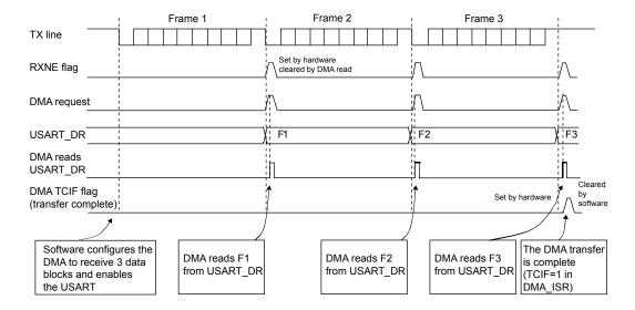
Figure 134. Reception using DMA
