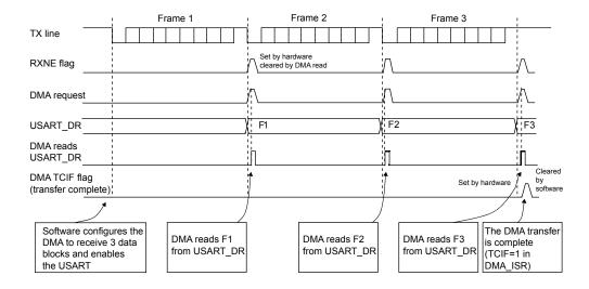
Figure 146. Reception using DMA
