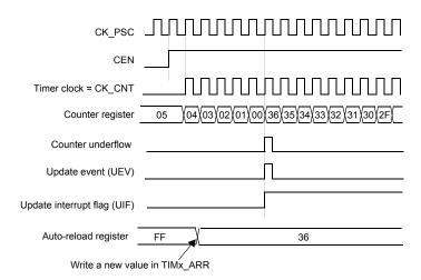
Note: Here, center-aligned mode 1 is used (for more details refer to Section 16.4: TIM1 registers).
