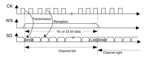
Data are latched on the falling edge of CK (for transmitter) and are read on the rising edge (for the receiver).
