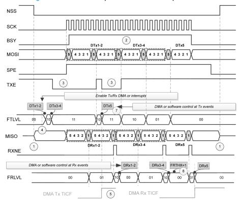
Figure 162. Master full-duplex communication in packed mode
