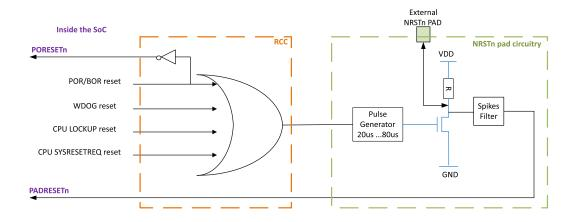
Note: The system reset information is output on the NRSTn pad to inform the external world and reset other elements on the board if needed.
