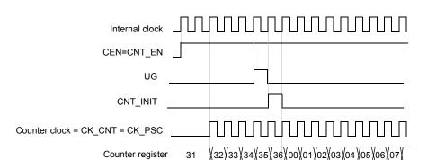
Figure 50. Control circuit in normal mode, internal clock divided by 1
