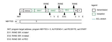
Example SMBus controller receiver 2 bytes + PEC, software end mode (RESTART)
