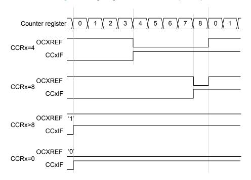
Figure 62. Edge-aligned PWM waveforms (ARR=8)
