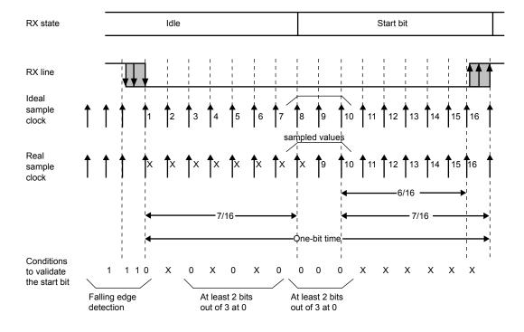
Figure 117. Start bit detection when oversampling by 16 or 8
