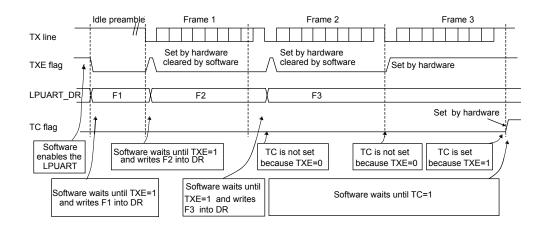
Figure 141. TC/TXE behavior when transmitting
