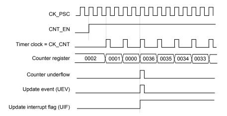
Figure 39. Counter timing diagram, internal clock divided by 4
