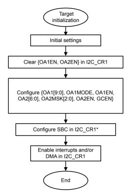
Figure 89. Target initialization flowchart
