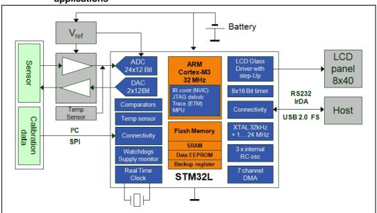
The proprietary mixed signal EEPROM technology used in the STM32L permits to integrate many of the components on a single chip leading to a reduction of the bill of material, and simplifying the power consumption and battery management.
