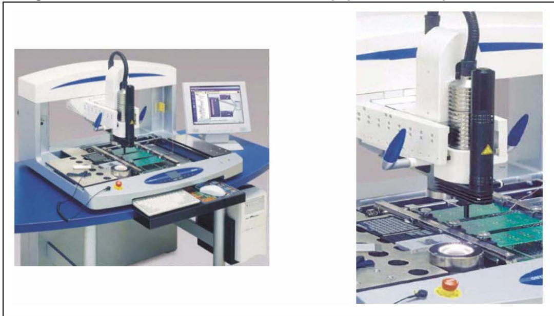
Figure 12. Comintec ONYX32 semi-automatic equipment for component rework
