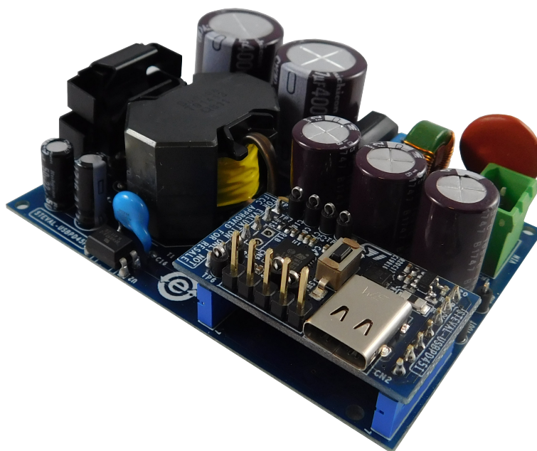
Figure 1. STEVAL-USBPD45C 45 W AC-DC adapter reference design kit
