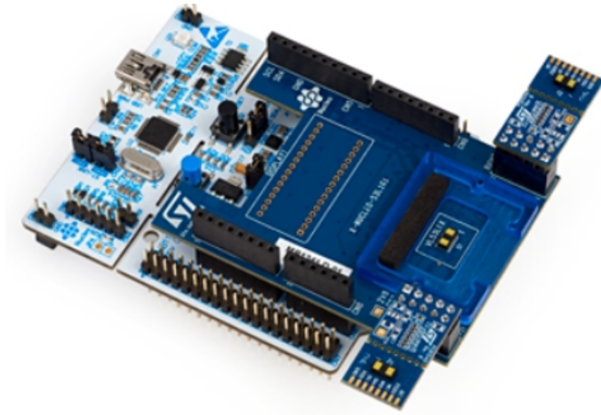
Figure 3. Breakout boards plugged onto the expansion board
