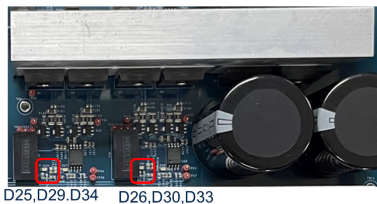
Figure 6. STDES-30KWRECT power board LEDs (2 of 2)
