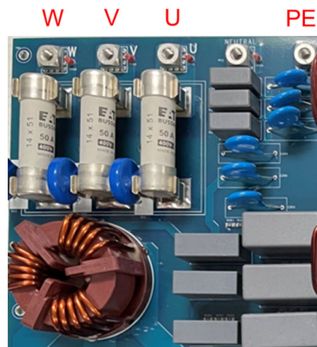
Figure 8. AC input wire connection
